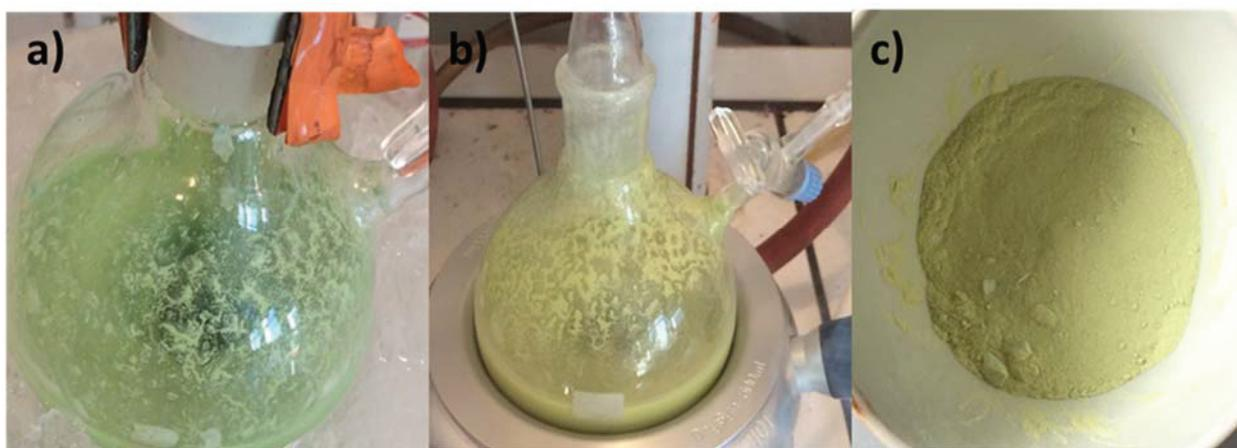
Figure 2-4: Color of the sample for the two steps method; a) in solution at 0°C, b) in solution at 60 °C and c) after drying
