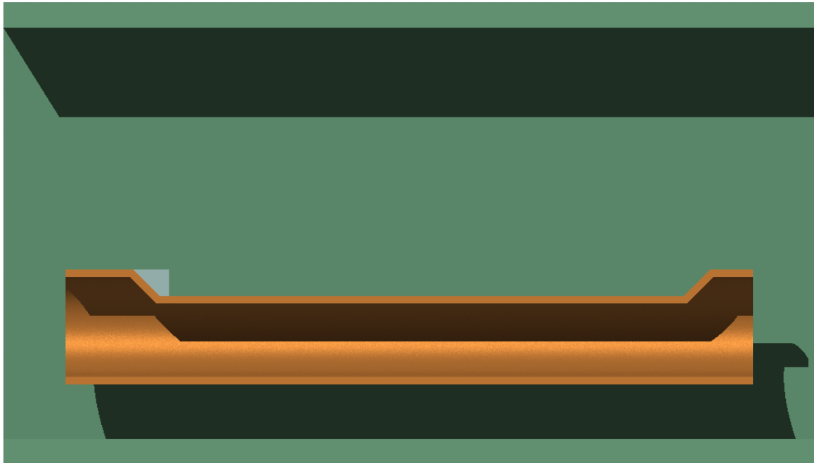
Figure 5.64: Geometry of the inclined window shaped beam pipe with a local leaded glass shielding box surrounding it.
