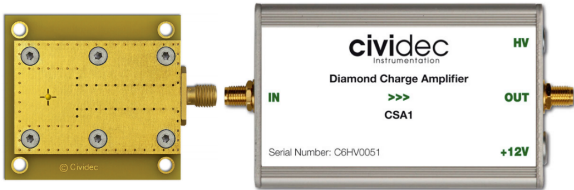
Figure 3.11: Diamond detector and fast charge amplifier bought from CIVIDEC [71].
