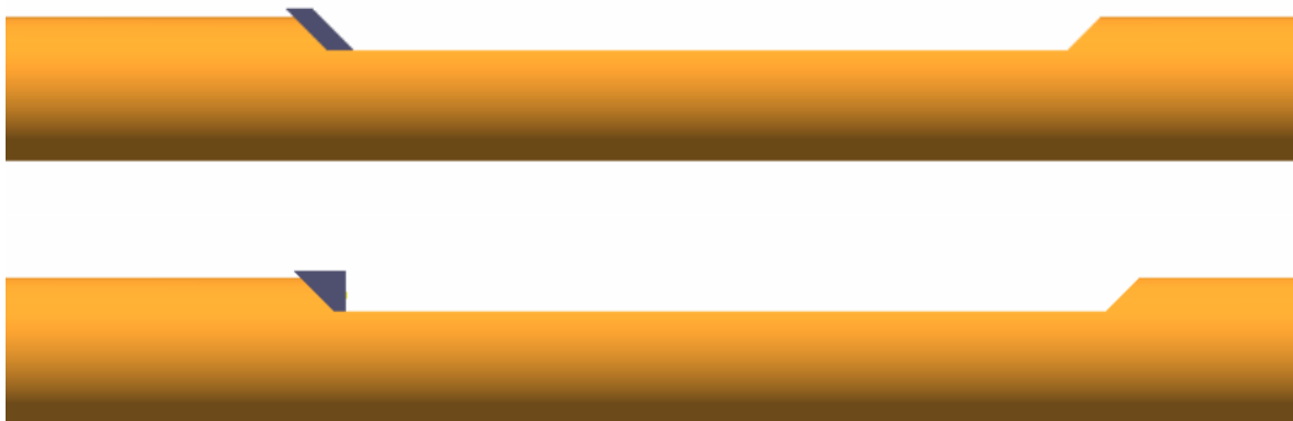
Figure A.7: Schematic of the Tungsten radiators (parallel above and trapezoid bottom) coupled with the 45° window shape beam pipe.
