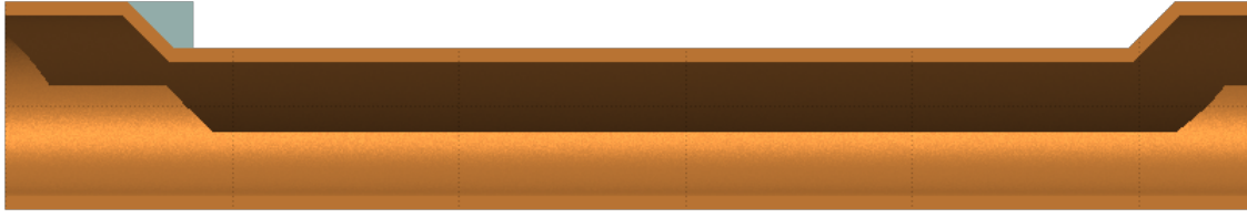
Figure 4.14: Geant4 model of the 45^\circ window shaped beam pipe coupled with a Tungsten radiator with effective thickness of 4 \times RL installed after the quadrupole QKBLP in LER.
