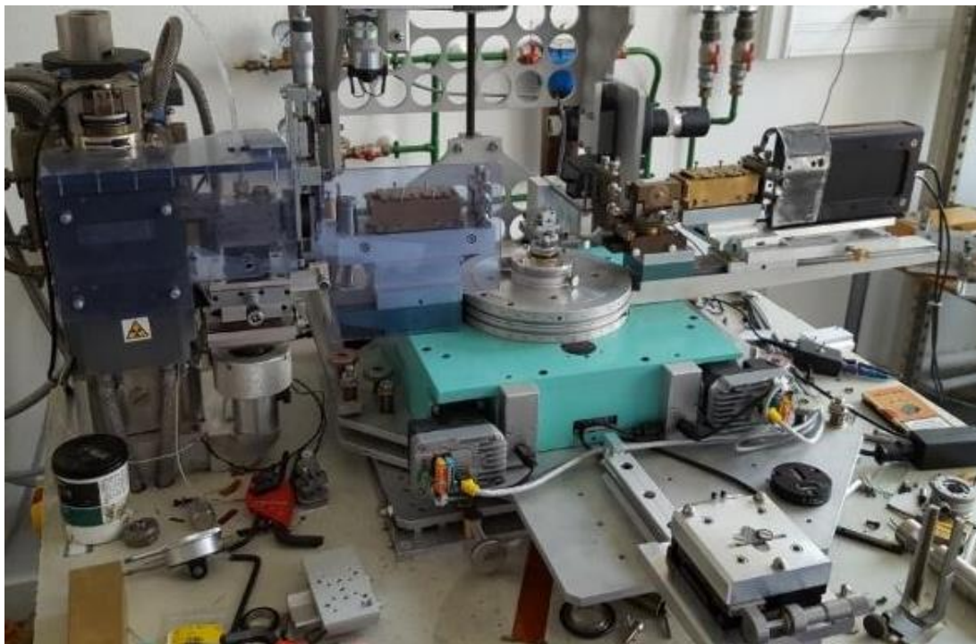
Figure 6. Home-made powder diffractometer (Gonio).
