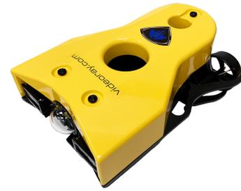
(e) VideoRay Pro 5 , launched in 2018. System of interchangeable, modular components. Forward speed: 4.4 *knots*. Weight: 10 *kg*. Depth rating: 305 *m*.
