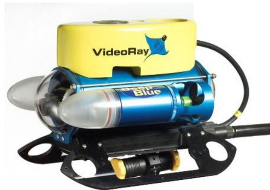
(d) VideoRay Deep Blue, launched in 2004. Enhanced depth rating up to 305 m. Featured a Tritech SeaSprite scanning sonar.
