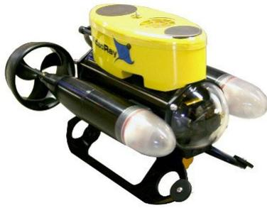
(a) VideoRay Pro 3 GTO, launched in 2005. More powerful thrusters allow increasing speed from 2.6 to 4.1 *knots*
