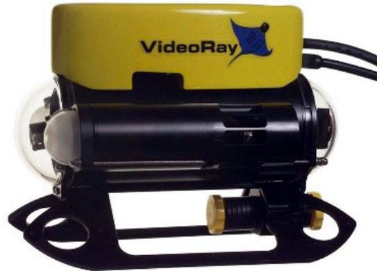
(b) VideoRay Pro II, launched in 2002. Added more 80% thrust, new lighting, enhanced hydrodynamic performance, upgraded camera and lowered power consumption.
