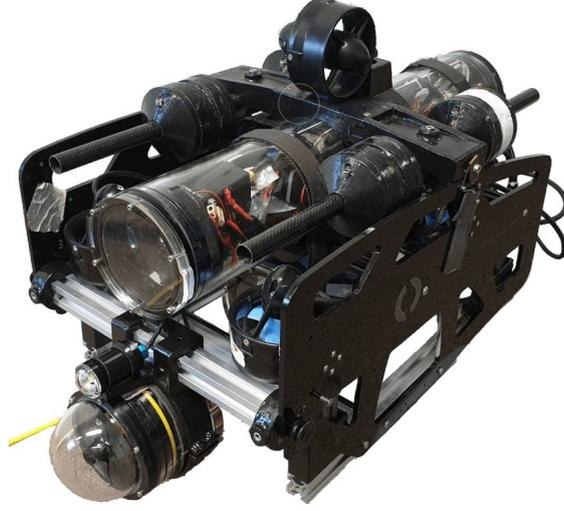
Figure 6.9: AUV with downward-looking camera
