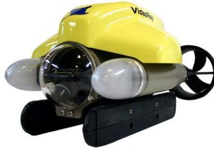
(b) VideoRay Pro 4 , launched in 2009. Improved hydrodynamic performance, camera and ballast adjustment. New control software platform for pilot. Increased vertical and horizontal thrust. Weight: 6.1 *kg*. Depth rating 305 *m*.
