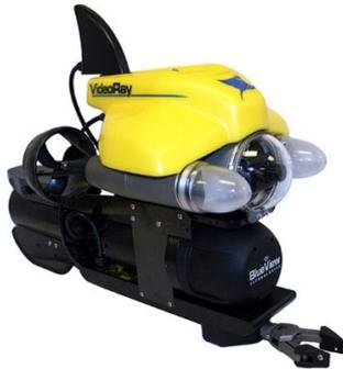
(c) VideoRay CoPilot by Seebyte, launched in 2012. Featured autonomous control. CoPilot provides effortless and automatic navigation to underwater locations all while following a pre-defined mission regardless of changing currents and rough sea conditions.
