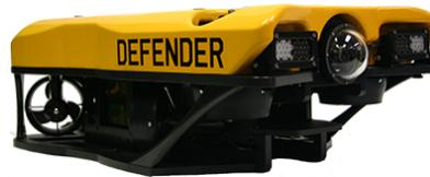
(d) VideoRay Mission Specialist Defender , launched in 2017. Modular design of platform allows easily customizable to adapt to specific missions. Depth rating: 1000 *m*. Weight: 17.2 *kg*.
