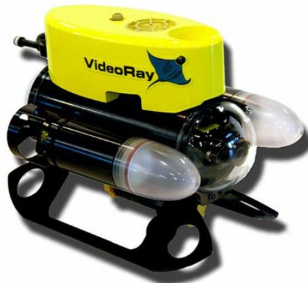
(c) VideoRay Pro 3, launched in 2004. Upgraded lighting, camera and thrusters. New 9-pin accessory plug for optional capabilities. Introduced control through a laptop PC which allow data can be gathered and analyzed.
