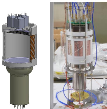
Figure 3.5 – Left panel: 3D drawing of the TPC. Right panel: picture of the TPC.
