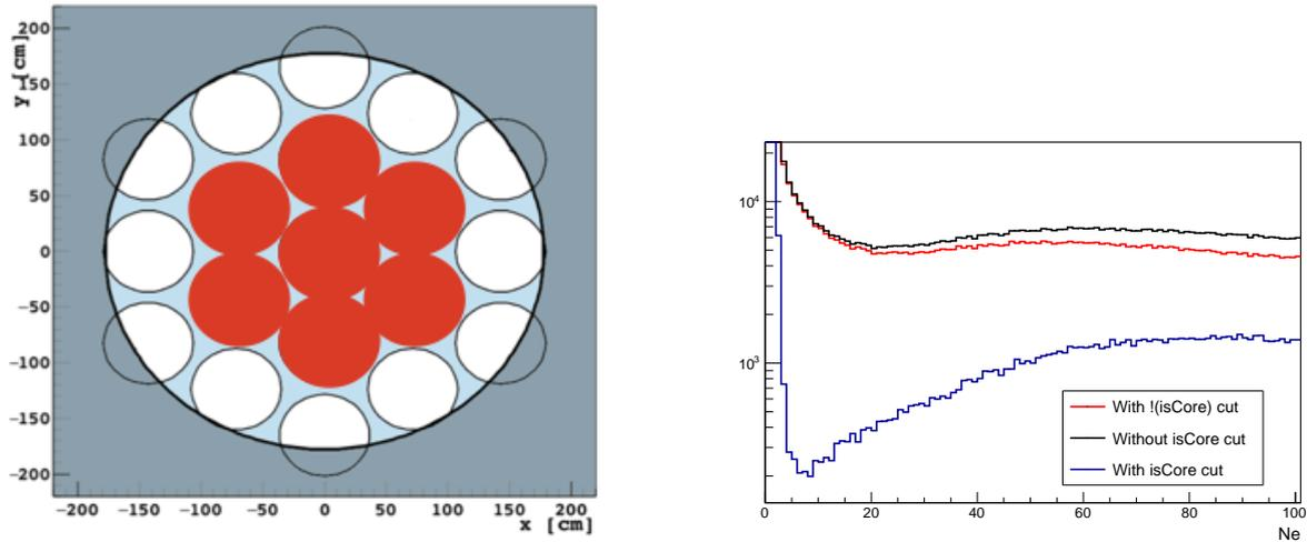
(a) Top PMT array of DarkSide-50. The red PMTs are the one requested to have the highest quantity of light for fiducialization.
