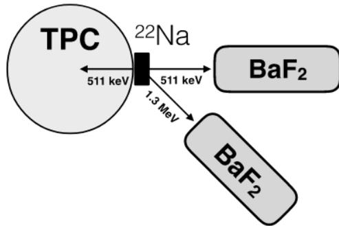
(a) Trigger efficiency measurement setup (top view).
