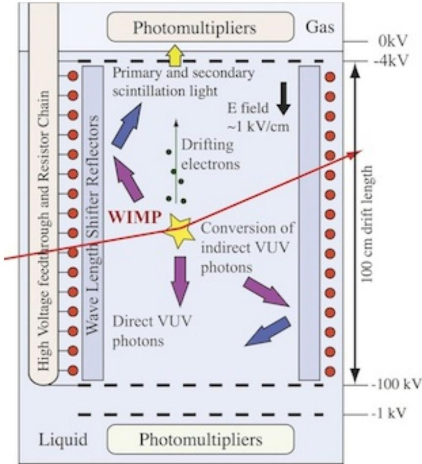
Figure 2.1 – Principle of a dual-phase TPC.
