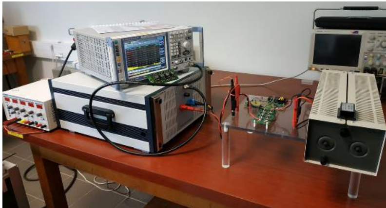
Figure IV-23 Disposition du test CEM final
