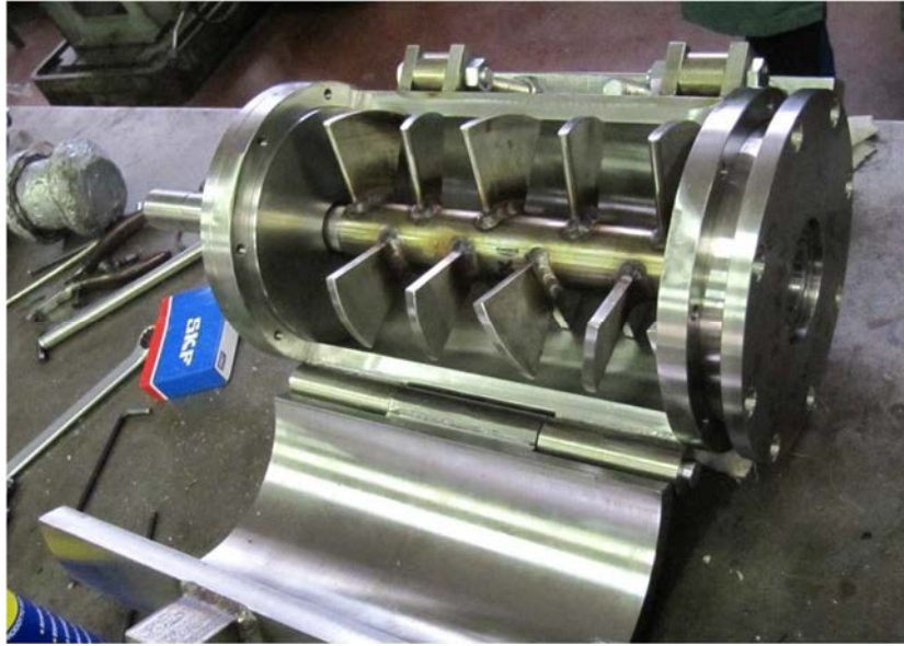
Figure 42: Cylindrical stator and rotor with blades of the turbomixer equipment.
