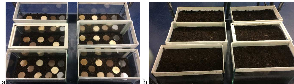
Figure 54: Samples have been placed over 1kg of soil (a) and then have been covered with another kg of soil to perform composting tests.
