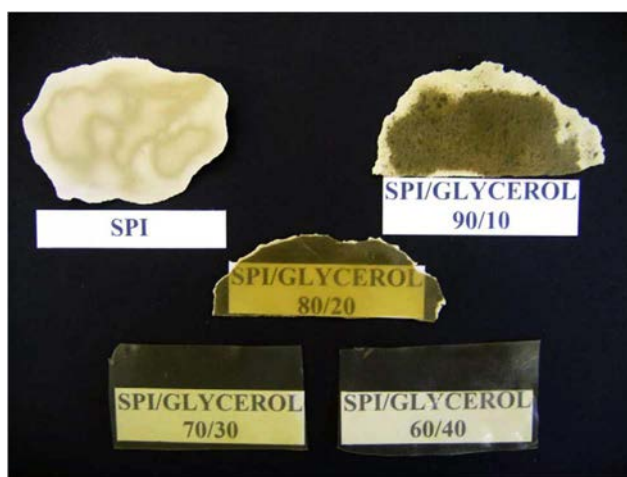
Figure 30: Different SPI films with 0-10-20-30-40 wt.% of Glycerol [ 59].
