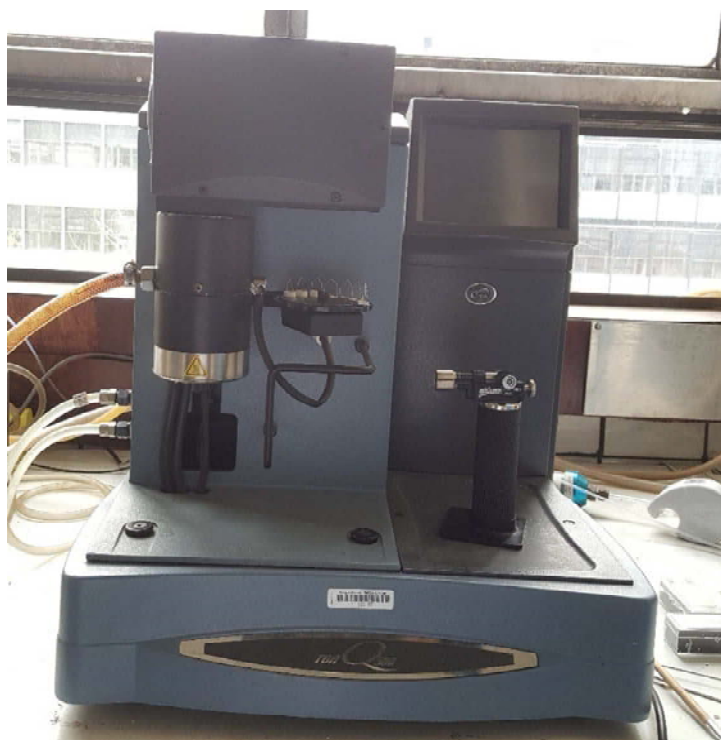
Figure 46: Thermogravimetric analysis equipment used to analyse thermal stability of our samples.
