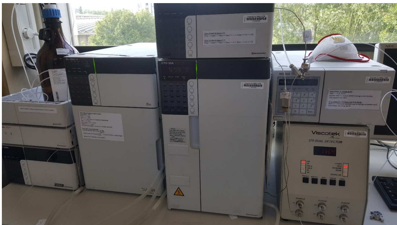
Figure 51: Size Exclusion Chromatography equipment used to evaluate molecular weight of PLA-based samples.
