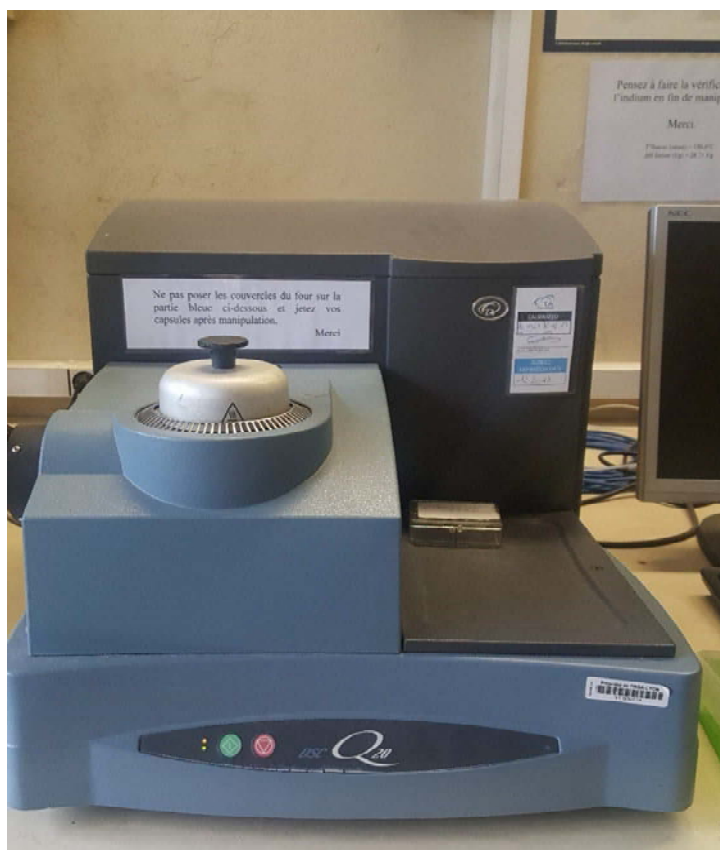
Figure 45: Differential Scanning Calorimetry equipment used to analyse thermo-chemical properties of samples.
