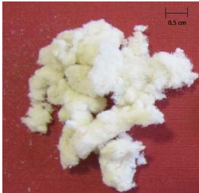
Figure 59: Recycled paper after micronizing process through Superfine grinding mill.
