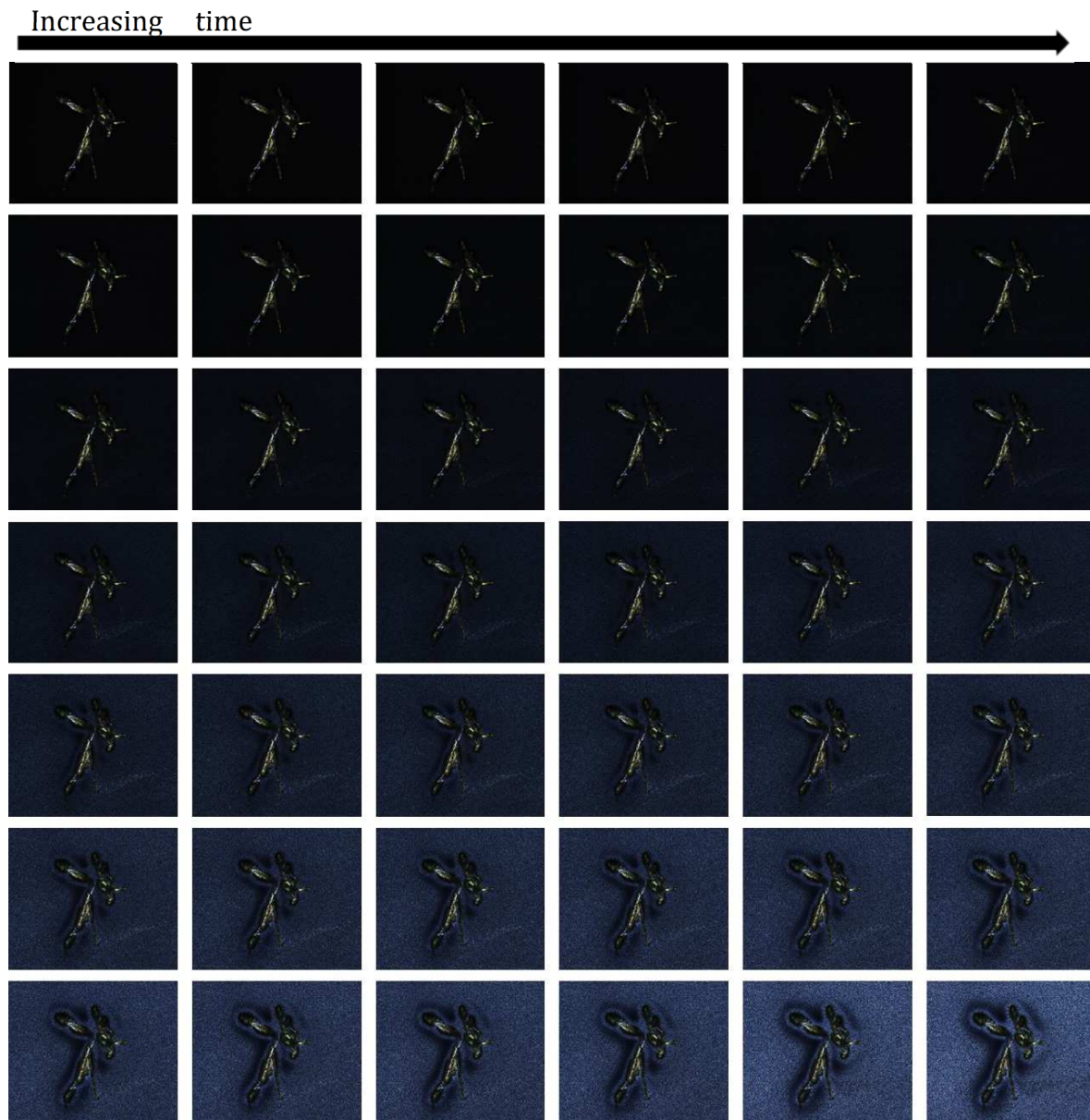
Figure 114: Crystals growth in PLA with wood flour (PLA60-WF40), studied with a thermo-optical microscope at 100X magnification with polarized light.
