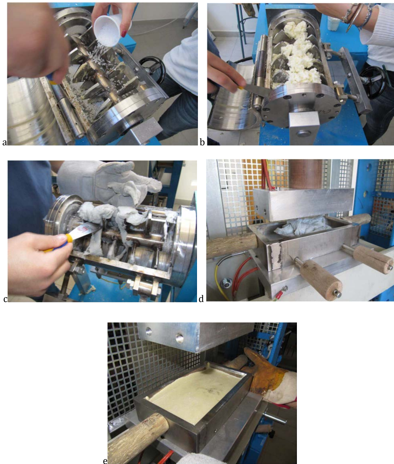
Figure 43: General process to obtain samples with turbomixer processing: a) Introduction of polymer pellets, b) Introduction of natural fillers, c) Extraction of the melted charge after processing at melting temperature and high speed rotation, d) Introduction of melted charge in the compression moulding equipment, e) Extraction of samples.
