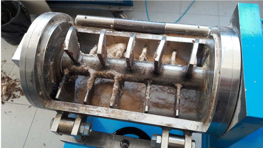
Figure 120: Tubomixer processing of samples with HDPE, PLA, wood flour and recycled waste paper.
