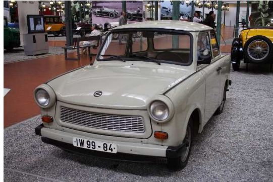
Figure 13: Trabant car, produced in 1958 in the German Democratic Republic with main parts made of composites with natural fillers [Wikipedia, Trabant, 18/11/2016]
