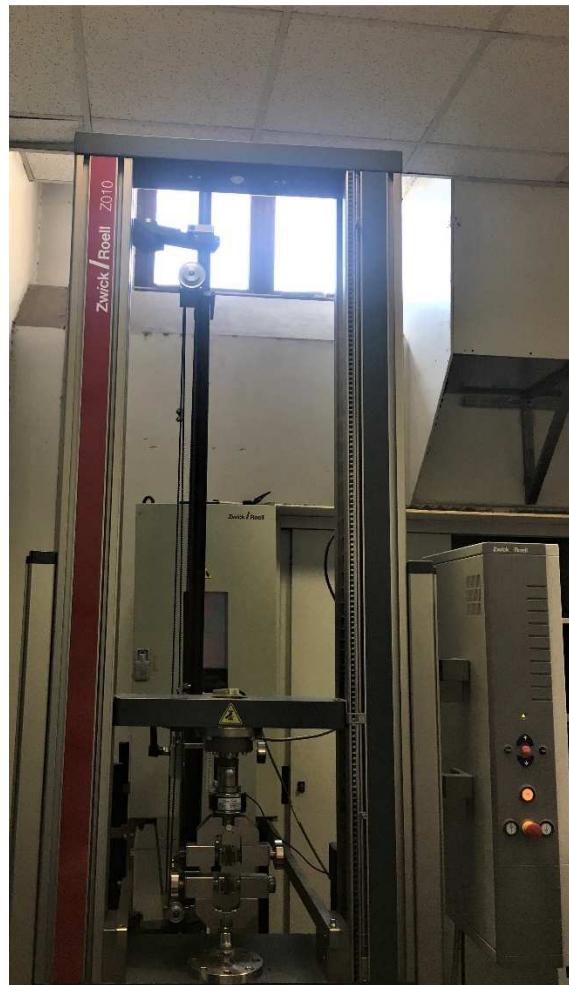
Figure 44: Tensile test equipment used to evaluate mechanical properties.
