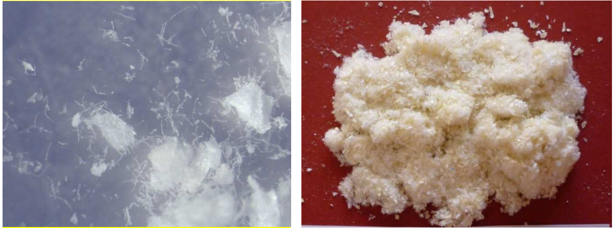
Figure 61: Stereomicroscopy image and visual observation of recycled paper after micronizing process through Knife mill.
