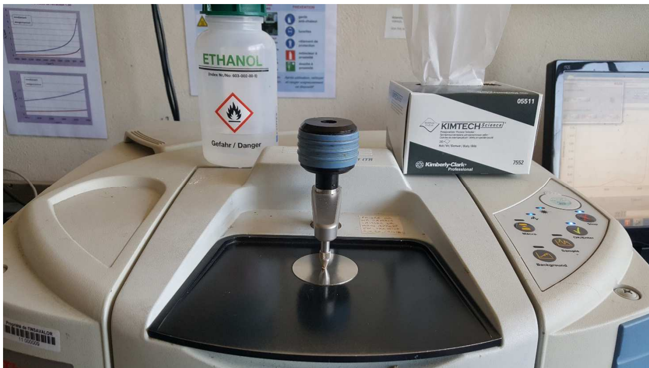
Figure 50: Infrared Analysis Attenuated Total Reflection (ATR-FTIR) equipment used to evaluate interactions or reactions between components.
