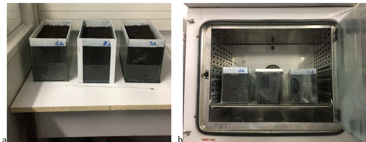
Figure 52: Aquaria used to perform composting tests at mesophilic (a) and thermophilic (b) conditions.
