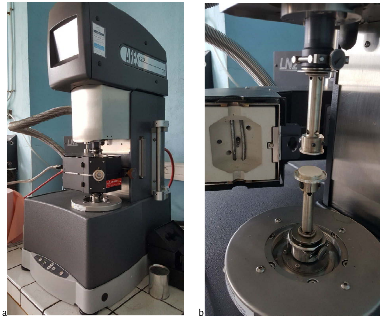
Figure 48: Rheology equipment used to perform rheological measurements.
