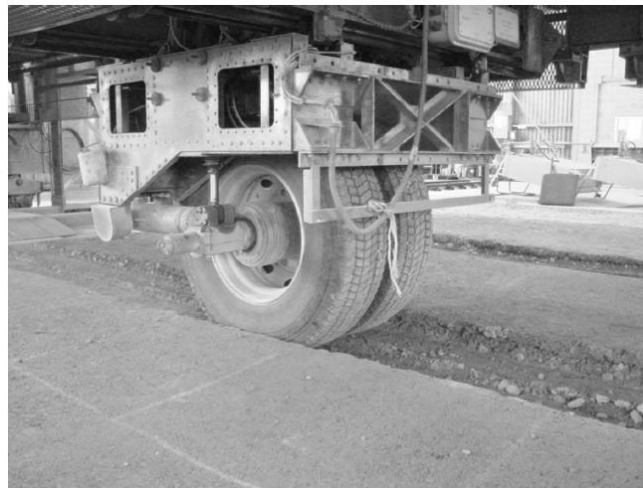
Figure 1.5-14: View of PTF carriage fitted with dual wheel assembly. (Cook et al., 2016)
