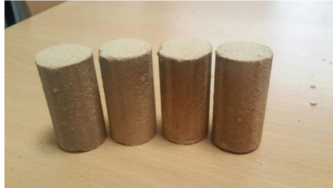
Figure 2.3-5: Triaxial prepared specimens.
