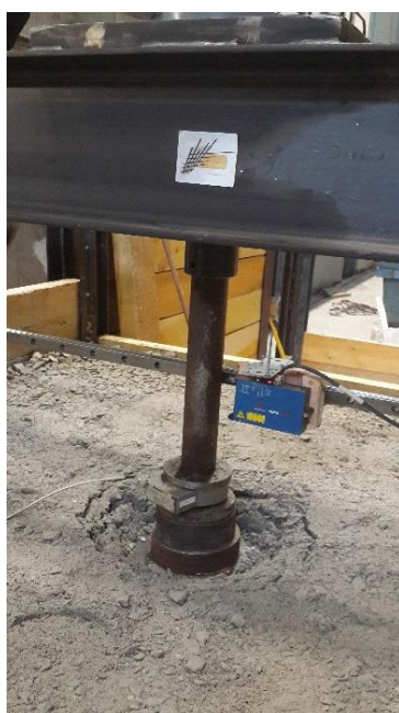
Figure 2.6-6: Laser sensor installation and measurements.
