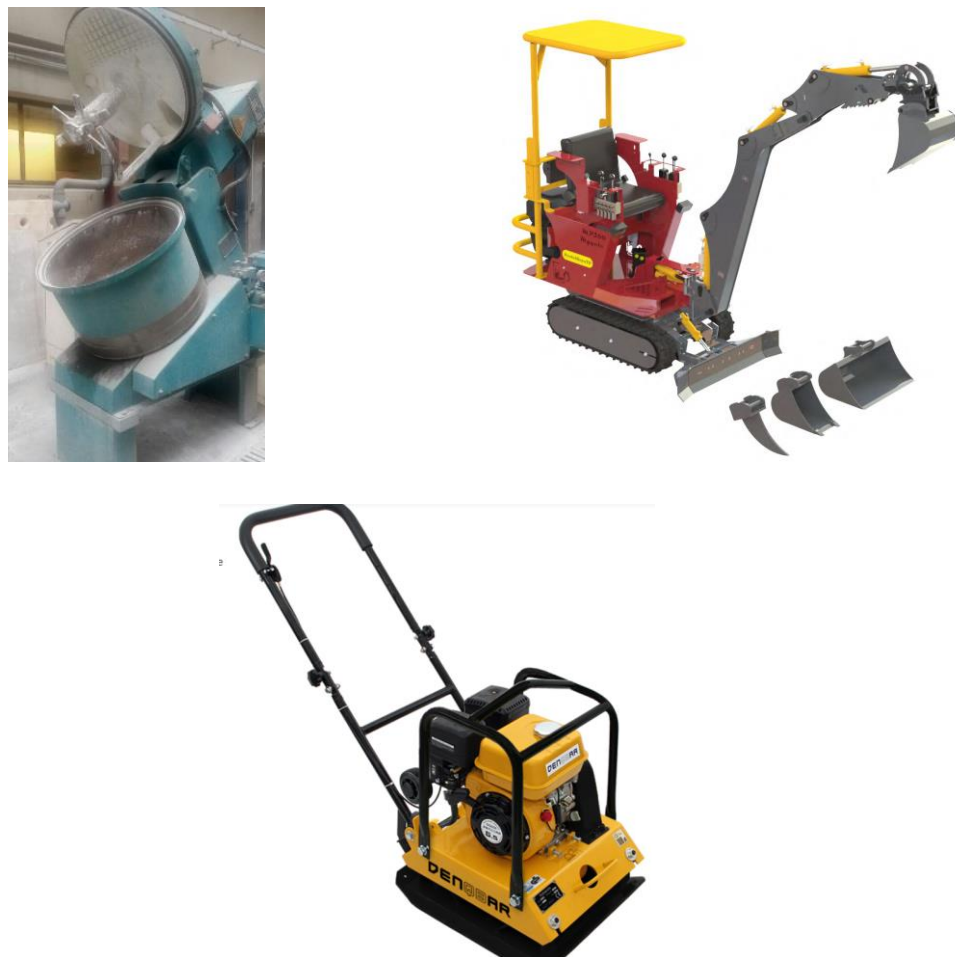
Figure 2.4-1: The mixer, plate compactor and mini excavator used for the soil installation.
