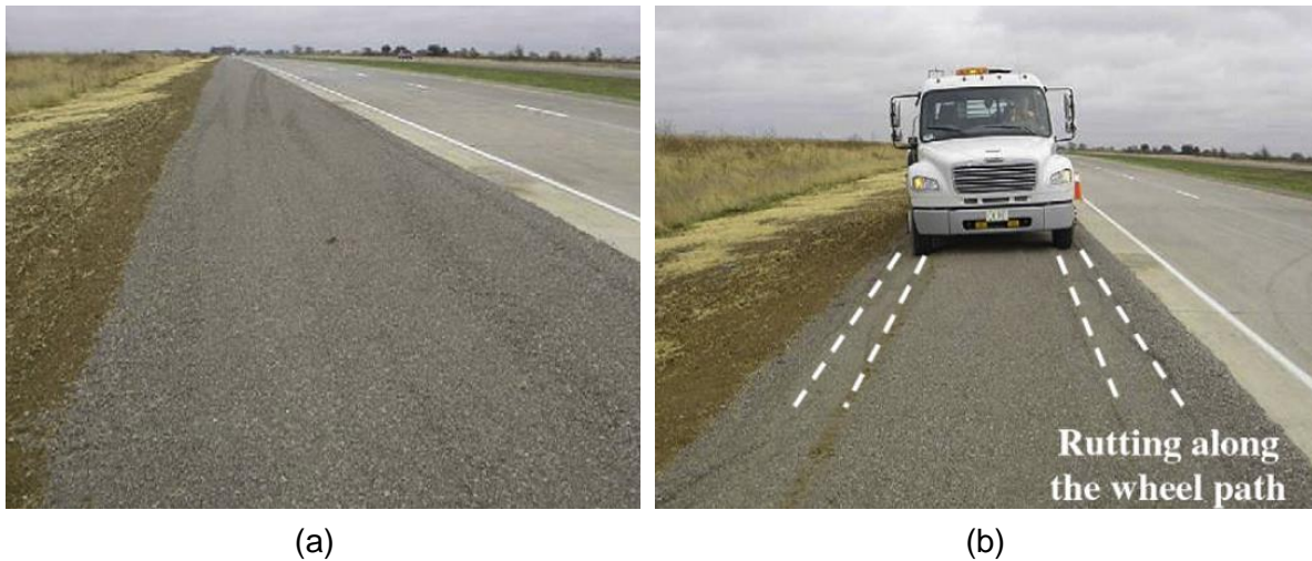
Figure 1.5-10: (a) Prepared testing sections, (b) 76 mm rut developed with few truck passes. (Mekkawy et al., 2011)
