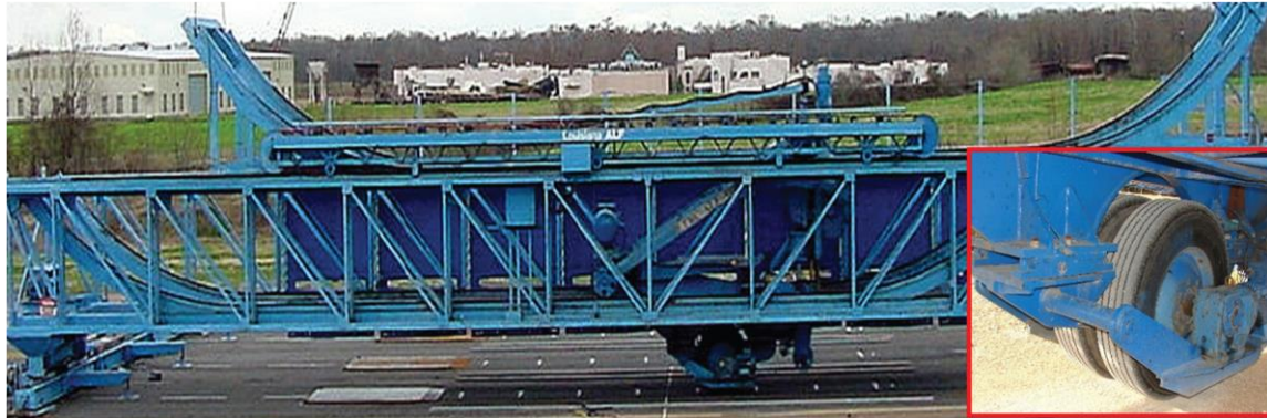
Figure 1.5-21: ALF with insertion of dual-wheel assembly. (Tang et al., 2015)
