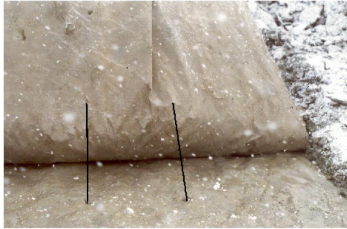
Figure 1.9-3: Example of geotextile punching. (Brady et al. 1994)
