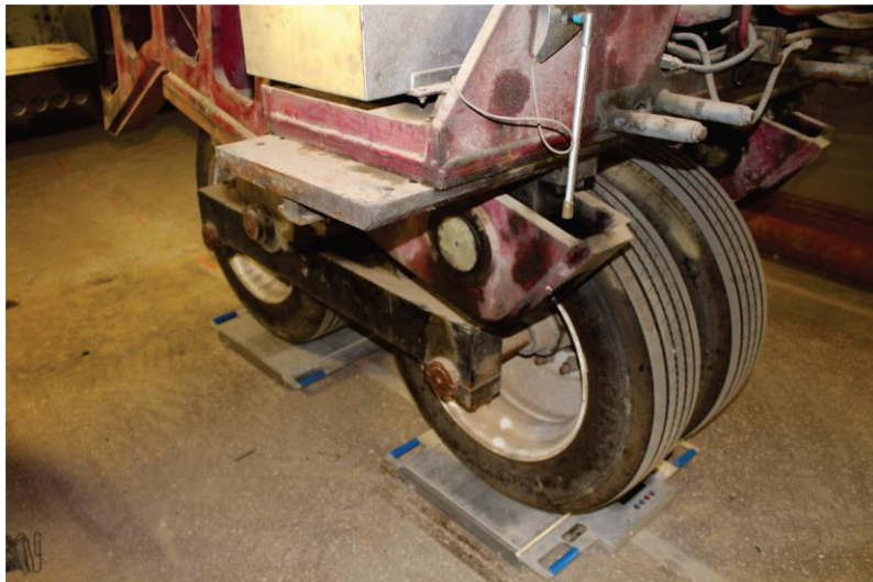
Figure 1.5-17: Dual-wheel tandem axle configuration. (Robinson et al., 2017)
