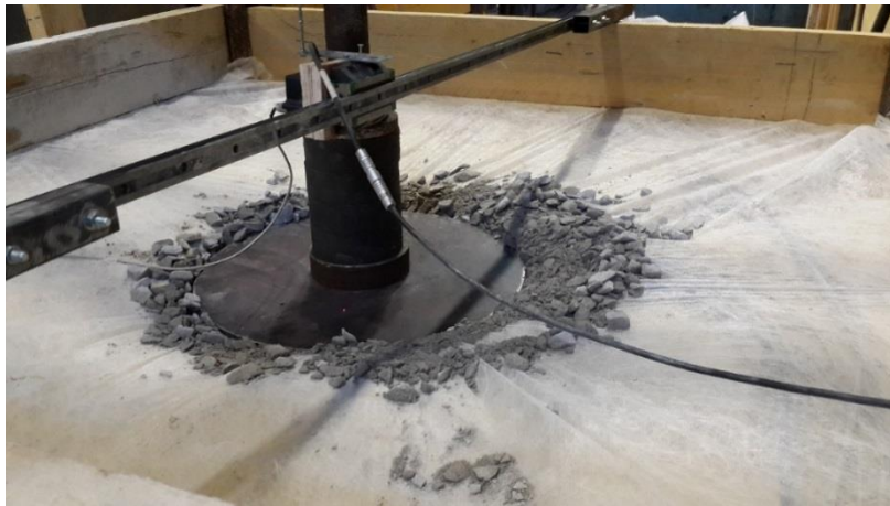
Figure 5.4-5: Plate load test performed directly on the subgrade soil.
