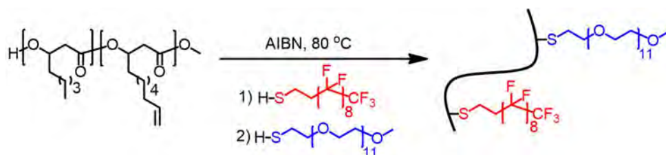
Scheme 1.35 Synthetic pathway for the preparation of functionalized fluorinated/PEG PHA.
