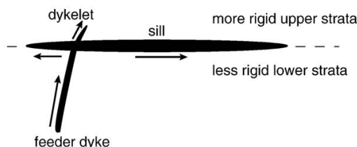
Fig. 2. Diagram illustrating the experimental observations of Kavanagh et al. (2006) for the formation of sills in layered elastic solids under lithostatic stress conditions. Sills were observed to form only when their feeder dyke intersected an interface separating a lower, less rigid layer from an upper, more rigid one. In some cases, a dykelet would protrude into the upper rigid layer, yet would always quickly stop propagating while the sill pursues its propagation. Arrows show the directions of propagation.
