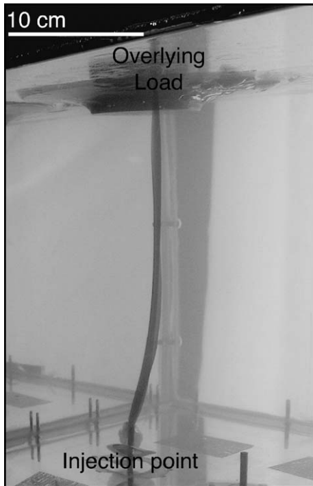
Fig. 3. Photograph of experimental dyke formation propagated with an overlying load (side view, at 909 s, Experiment 12). The load acts as an attractor to dyke propagation.
