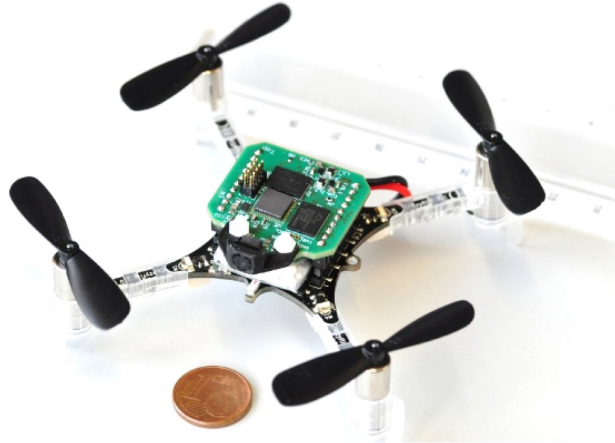
Figure 1.21 – Crazyflie with a GAP8 microcontroller on top of it for autonomous navigation. Image.
