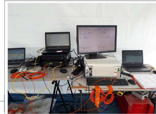
d - DTS units installed in the field
