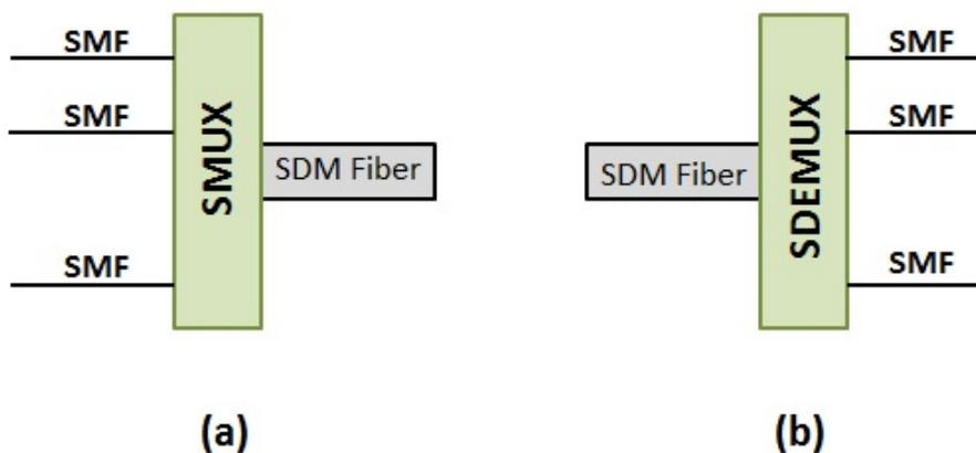
Figure 1.15: Spatial multiplexing and demultiplexing scheme
