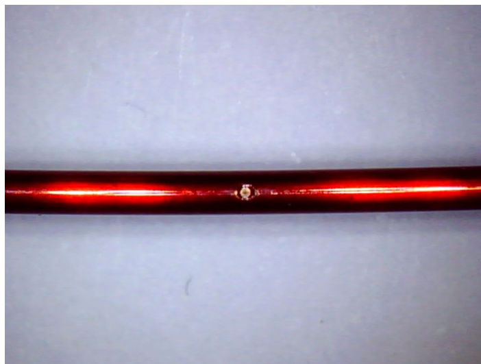
Figure IV.1: Photograph of a broken specimen made of APX-1 (CV).
