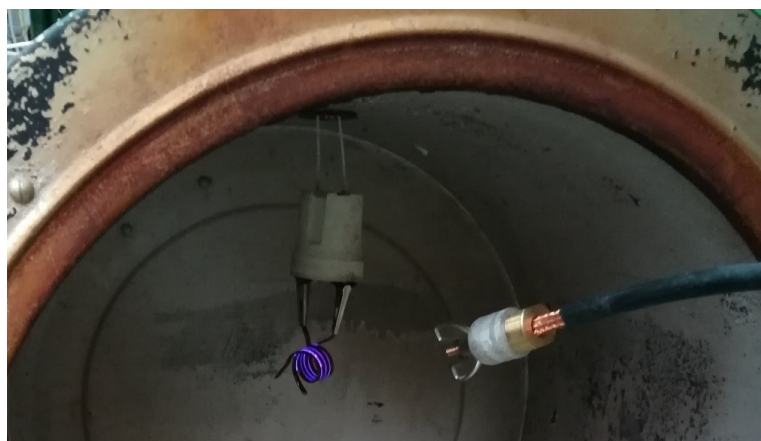
Figure III.34: Photograph of antenna detecting PD on the coil tested under high dV/dt impulse voltage V_{dc} = 1.4 \text{ kV} , f = 50 \text{ kHz} .
