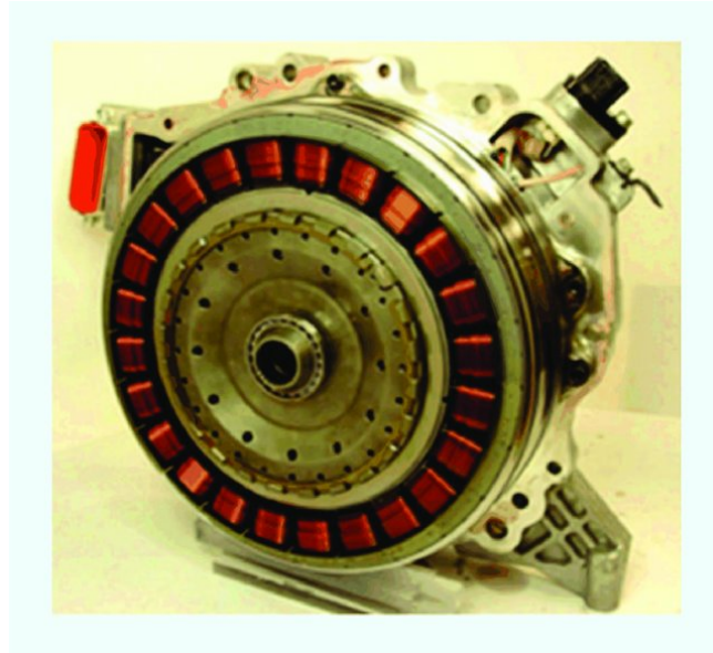
Figure I.17: Concentrated winding configuration of a Hyundai Sonata 2011 motor [66].
