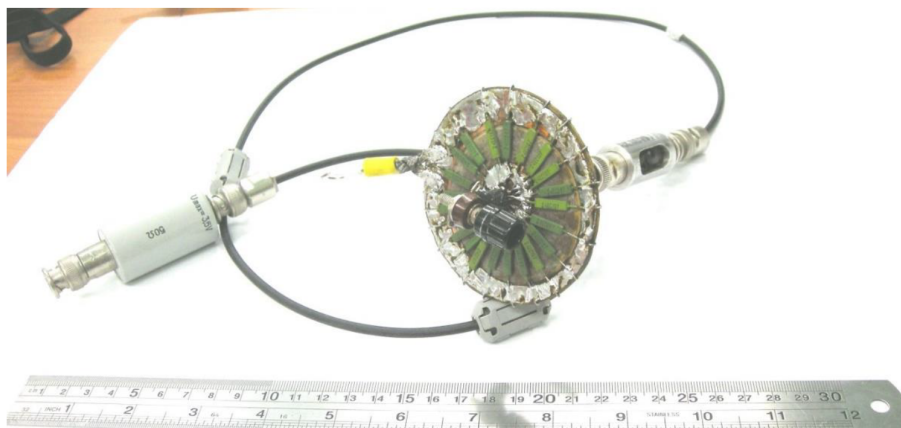
Figure 4: Photograph of current shunt.
