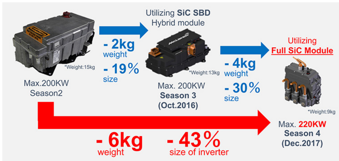
Figure I.5: Si and SiC inverters comparison [44].
