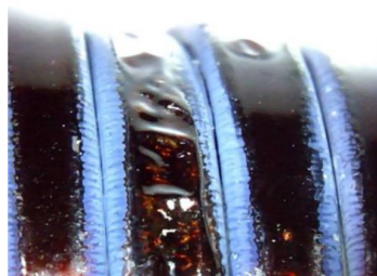
Figure IV.27: Microscopic images of rectangular winding wire after testing under high dV/dt impulse voltage, T=180^{\circ}\text{C} , f_s = 20\text{ kHz} , V_{dc} = 1.2\text{ kV} .
