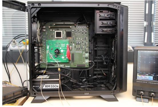
Figure 6.1: Stellar [80] hardware platform (with an embedded Virtex-7 FPGA)
