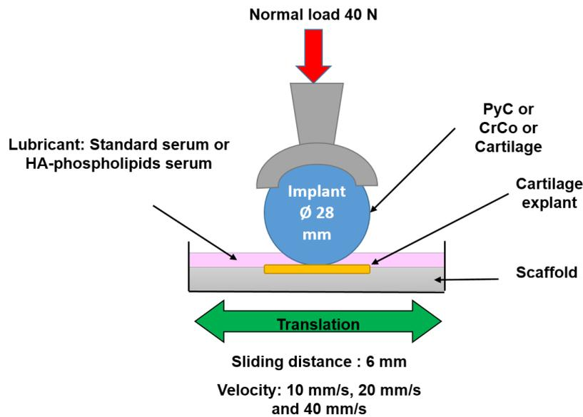
Figure F-4 schema of the friction test set-up
