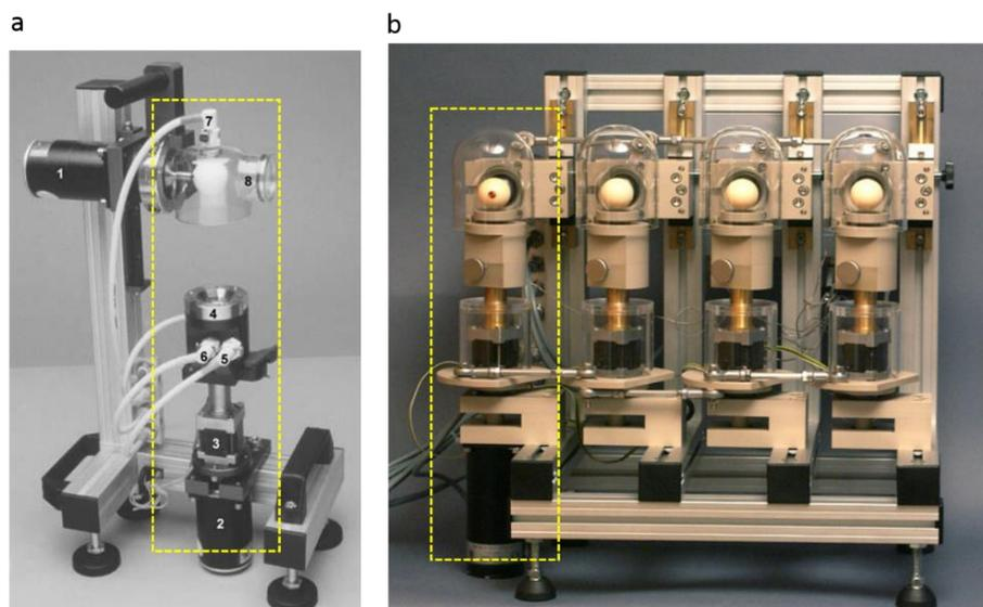
Figure F-7 a) One station configuration of the simulator: (1 and 2) step engines providing reciprocating motion for scaffold and of the ball, (3) actuator providing the compression, (4) cartilage sample holder. (Figure is taken from [206]), b) the final four-station set-up of the simulator
