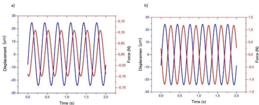
Figure G-9 Obtained signals with a displacement of 50 μm and a frequency of 3 Hz: a) Applied displacement and obtained force-displacement signals of the bee-honey, phase shift  $\pi/2$  b) applied displacement and obtained force signals of the synthetic HEMA, phase shift  $\pi$
