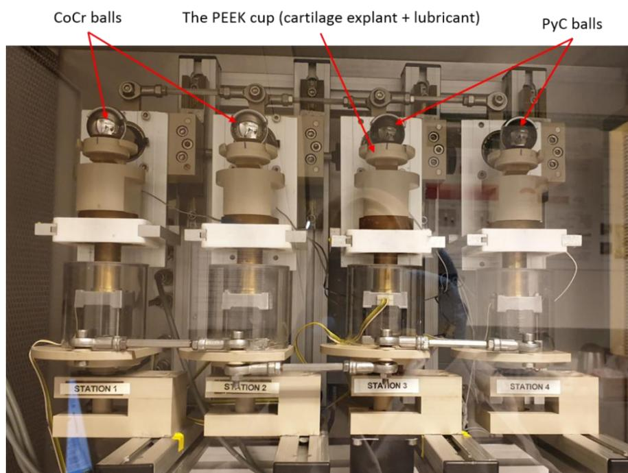
Figure F-9 the simulator set-up with CoCr and PyC balls housed in a controlled incubator (95 % humidity, 5 % CO<sub>2</sub>, 37 °C)
