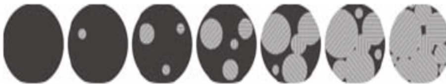
Figure 5.17: Amorphous bit (black) with a crystal nucleus (gray) progressively growing (from left to right) due to a laser beam that increases temperature inside the amorphous bit. Due to crystal growth, the amorphous bit becomes almost completely crystallized. Nevertheless polycrystallinity is observed, caused by the different orientations of the crystalline nuclei. Taken from: [42]
