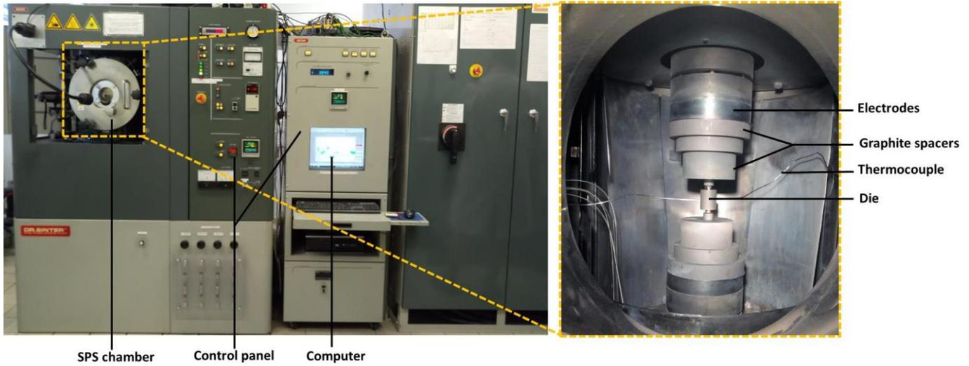
Fig. 2.2 SPS equipment: Dr. Sinter 2080 unit (SPS Syntex Inc., Japan)
