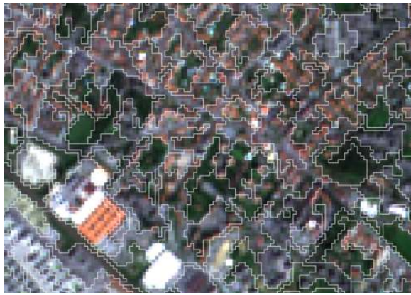
(a) First date of the Sentinel-2 time series overlaid with the SLIC segmentation at a scale of 10.
