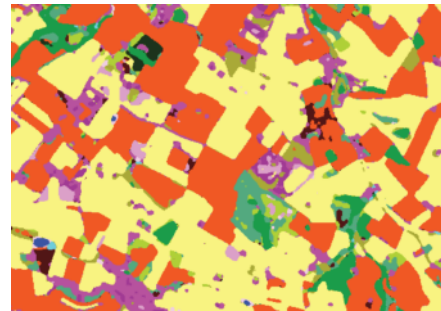
(b) Regularization in a 3x3 sliding window. The geometry remains relatively well respected, although some corners are slightly smoothed out.
