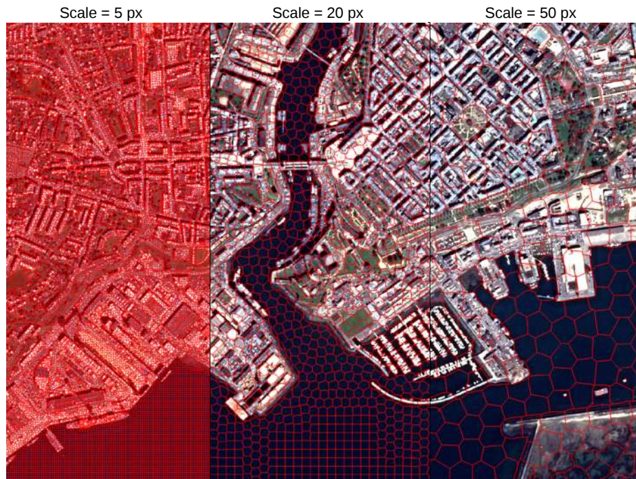
Figure 4.5: SLIC segmentation over Brest. The spatial width parameter offers control on the average size of the superpixels, which allows for a contextual description at a fixed scale. The illustration shows 3 scales of superpixel: 5, 20, and 50 pixels. These indicate the size of the initial grid used by the SLIC algorithm. In the segmentations, each superpixel contains in average 25, 400, and 2500 pixels.
