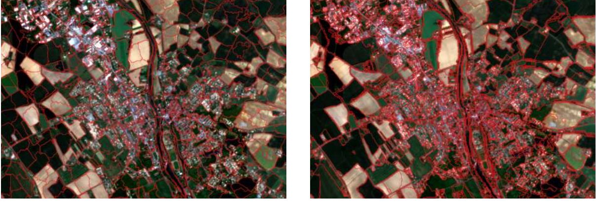
(a) SLIC superpixels. In the textured area, superpixels group together diverse pixels, and are therefore able to describe the density of the urban cover.
