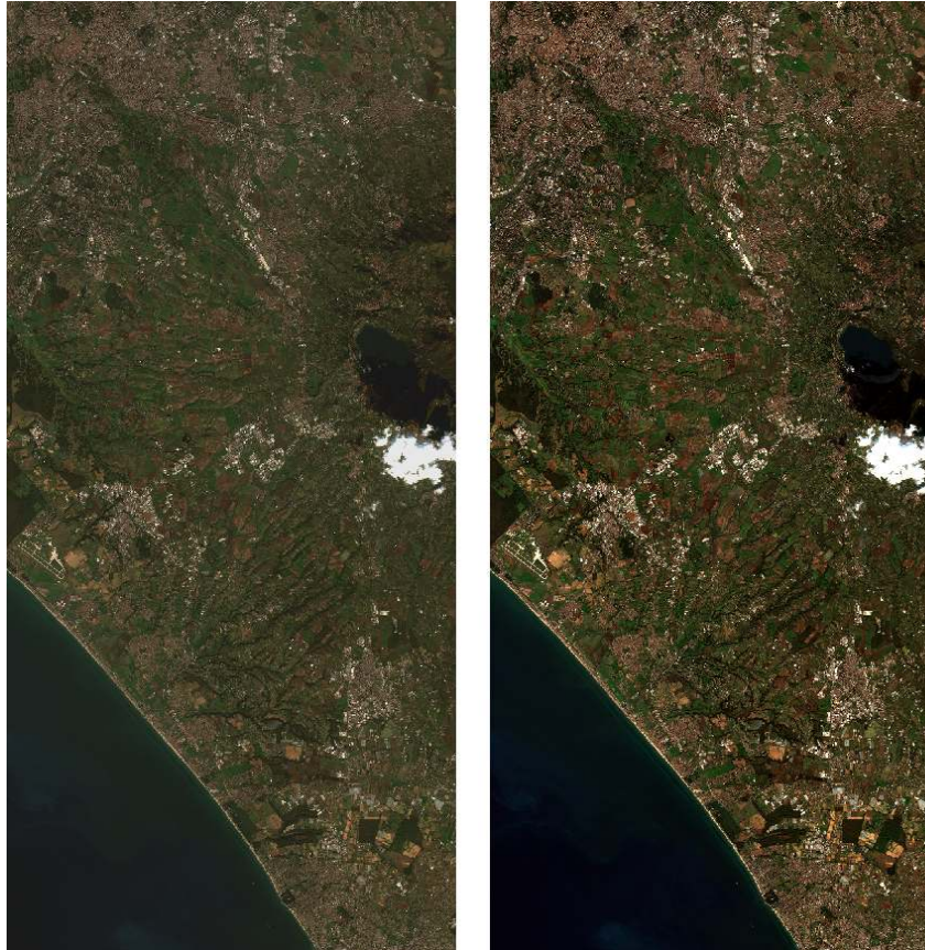
Figure 2.5: Left: The image of TOA reflectance is slightly lighter due to the presence of aerosols and water vapor in the atmosphere. Right: The image after atmospheric correction represents the BOA reflectance, in other words, the true reflectance at the surface of the Earth.
