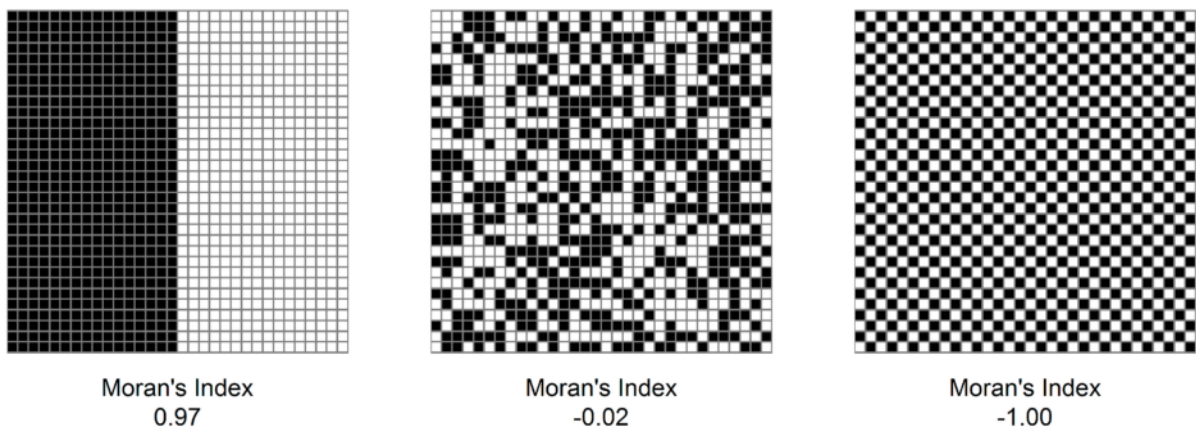
Figure 5.3: Illustration of Moran's index in three cases. In the first case, there is a strong amount of auto-correlation, in other words, neighboring pixels have a strong chance of being similar. In the second case, the pixels are randomly distributed, and the Moran's index is near zero. Finally, if there is a negative auto-correlation, neighboring pixels have strong chances of being different, which indicates a particular kind of texture.
