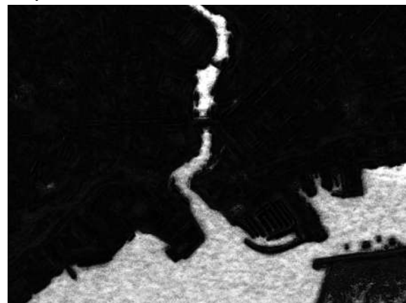
(f) Standard deviation of the histogram. It presents strong values for objects with an elongated shape.
