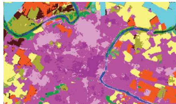
(h) Pixel and edge density features, in a Mean Shift object. The urban classes are more precise than with local statistics.
