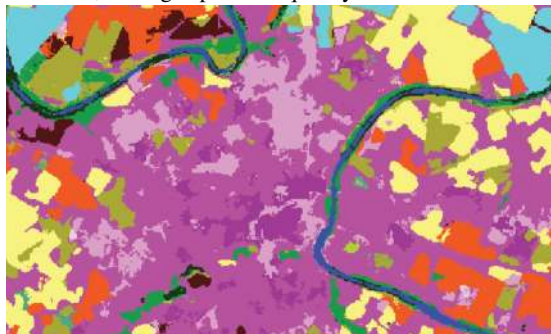
(e) Pixel, mean and variance features, in a superpixel of average size 100. Intra-object classification noise is reduced without altering the high spatial frequency areas.
