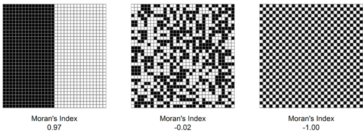
Figure 5.3: Illustration of Moran's index in three cases. In the first case, there is a strong amount of auto-correlation, in other words, neighboring pixels have a strong chance of being similar. In the second case, the pixels are randomly distributed, and the Moran's index is near zero. Finally, if there is a negative auto-correlation, neighboring pixels have strong chances of being different, which indicates a particular kind of texture.
