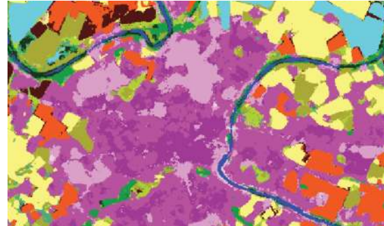
(d) Pixel and edge density features, in a sliding window of size 11x11. Some corners are preserved, but some are rounded.
