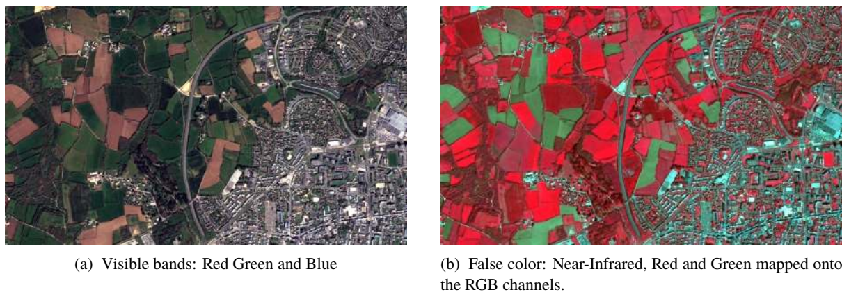
Figure 1.3: SPOT7 imagery at a 1.5m spatial resolution, over an area near the city of Brest. In the false color image, the Red band is replaced by the Near-Infrared band, the Green band by the Red band and the Blue band by the Green band. Infra-red is strongly reflected by vegetation, causing it to appear in shades of red.
