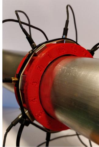
Figure 3.2: Transducers placed in the ring to maintain spacing.
