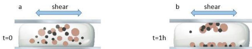
**Figure 2.** Schematic illustration showing the application of mechanical shear on the binary NR-CB suspension (a) and the formed coagulum (b).
