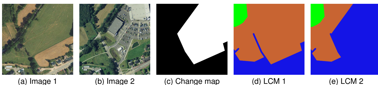
Figure B.1: Example of data that can be found in the HRSCD dataset. Coregistered aerial image pairs, change maps, and land cover maps contain semantic information about how the terrain has evolved over a period of six years.
