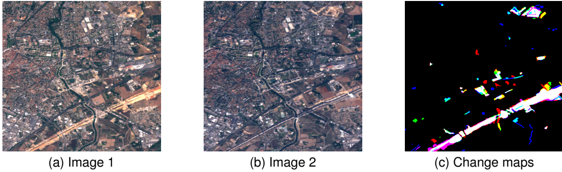
Figure A.2: Pair of coregistered images from the OSCD and manual change maps created by three different people. In (c), each colour channel contains the change map produced by a different person.
