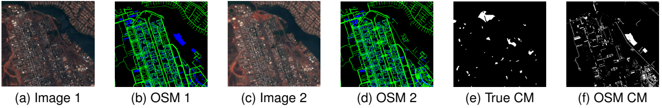
Figure 3.4: Comparing the OpenStreetMap semantic maps (b) and (d) relative to the images (a) and (c) leads to a change map (f) that does not resemble that which is produced by visual analysis (e).
