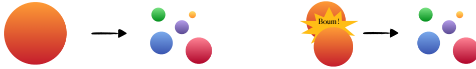
Figure 2.2: Left: Scheme of the spontaneous (or linear) fragmentation process of a particle of mass x into several smaller particles of mass y < x . Right: Scheme of the collisional (or non-linear) fragmentation process. Two particles of mass x and y collide and form several smaller particles of mass z < x + y .
