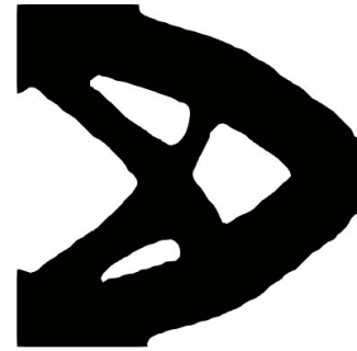
Figure 3.8: Resulting shape V_{max} = 0.95V^0 V/V^0 = 0.982655
