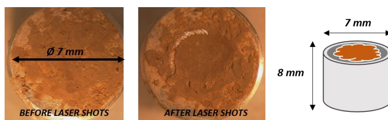
Figure 60 : Pictures of the Titan's Tholins powder pressed onto the indium sample-holder of the LAb-CosmOrbitrap before laser shot (left) and after laser shots (middle). On the middle picture, laser shots are visible on the brown Tholins powder, demonstrating the ablation of the sample. The scheme (right) illustrates dimensions of the sample-holder (8 mm height and 7 mm diameter).
