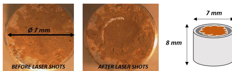
Figure 60 : Pictures of the Titan's Tholins powder pressed onto the indium sample-holder of the LAb-CosmOrbitrap before laser shot (left) and after laser shots (middle). On the middle picture, laser shots are visible on the brown Tholins powder, demonstrating the ablation of the sample. The scheme (right) illustrates dimensions of the sample-holder (8 mm height and 7 mm diameter).
