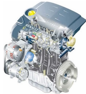
Figure 9.2: Reference engine (belt, accessories and bracket are in the lower left-hand corner)
