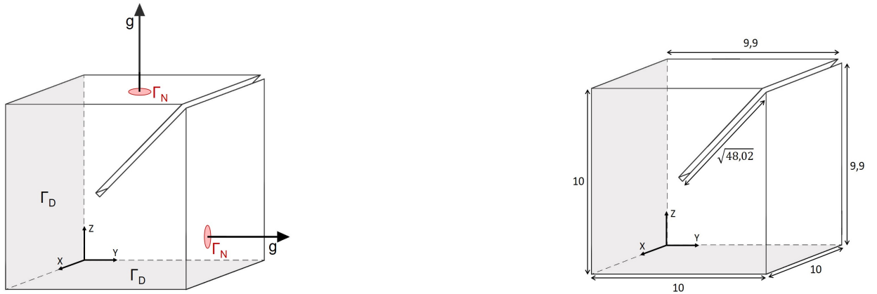
Figure 6.8: Cube with a slit, its loadings and dimensions
