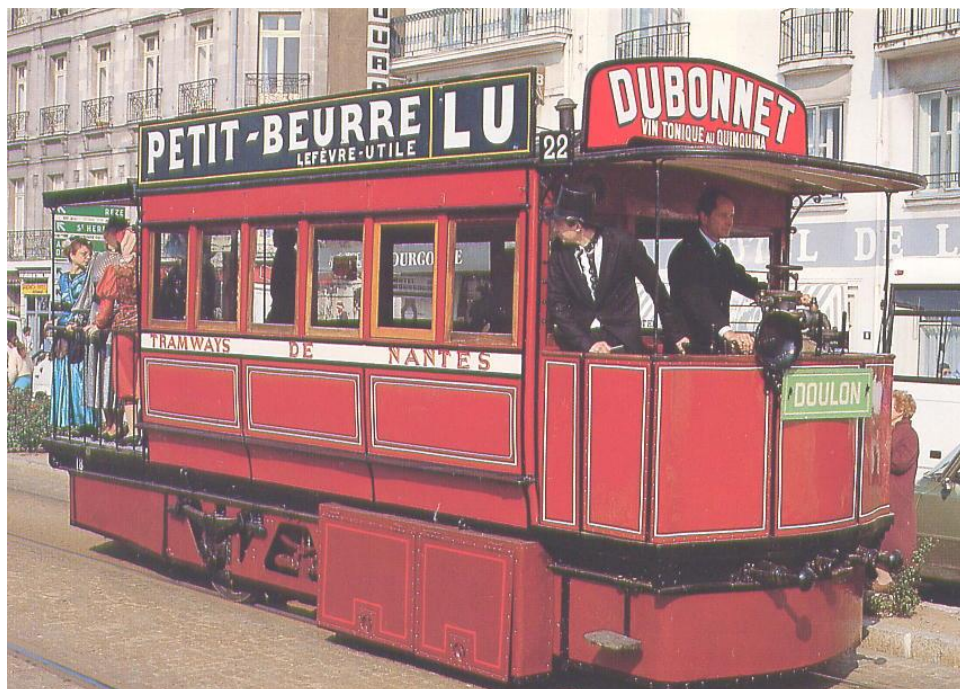
Figure 1.9: Mékarski compressed air system motor – Tramway Nantes [17]
