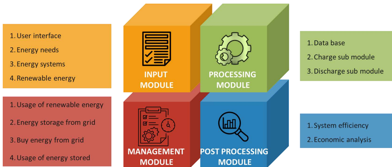
Figure 2.14: 3D matrices representing the main and sub modules of EXCEL VBA code
