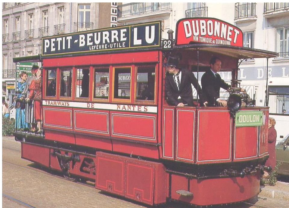
Figure 1.9: Mékarski compressed air system motor – Tramway Nantes [17]
