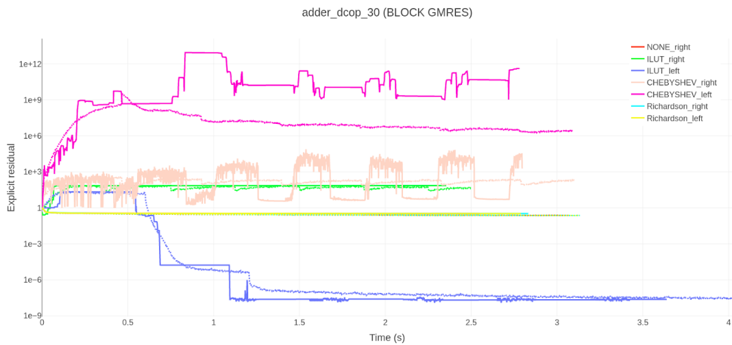
Figure 9.8: Convergence profile of all preconditioners with Block GMRES on the adder_doop_30 problem.
