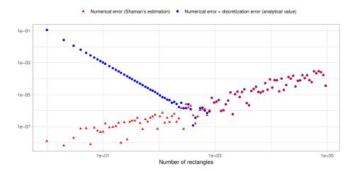
Figure 1: Integrating the cosine function between 0 and  $\frac{\pi}{2}$  using the rectangle rule. Both axes are displayed on a logarithmic scale. The analytically computed total error, discretization error plus numerical error, is plotted in blue, while our estimation of the numerical error is plotted in red. As the number of rectangles increase, the discretization error converges toward zero, leaving us with the numerical error due to the sum of areas.
