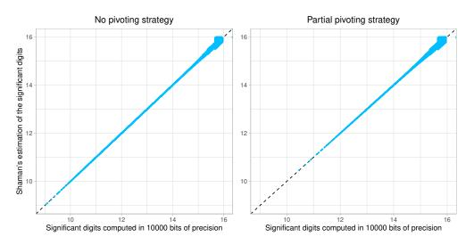
Figure 6.1: Estimation of the number of significant digits for the LU factorization algorithm computed in double precision. Each dot corresponds to a cell in the non-zero half of either the L or U matrix produced by the decomposition. The dashed line represents the equality between both estimations of the number of significant digits.
