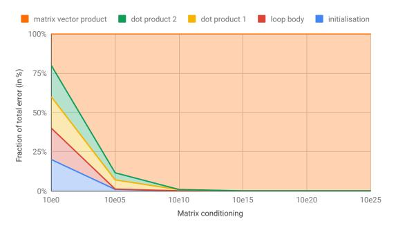
Figure 6.5: Distribution of the numerical error in the output of the conjugate gradient algorithm, in percents of the total error.
