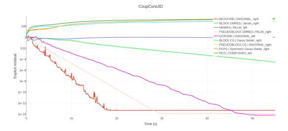
Figure 9.2: Convergence profile of a random selection of linear solvers and preconditioners for the CoupCons3D problem. The relative residual is displayed on a log scale.
