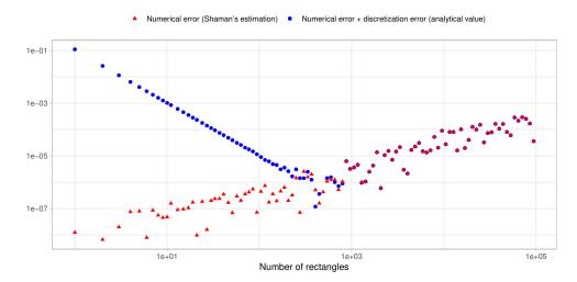
Figure 6.2: Absolute value of the error as a function of the number of rectangles used for the integration of the cosine function between 0 and  $\frac{\pi}{2}$  using the rectangle method. Both axes are displayed in a logarithmic scale.
