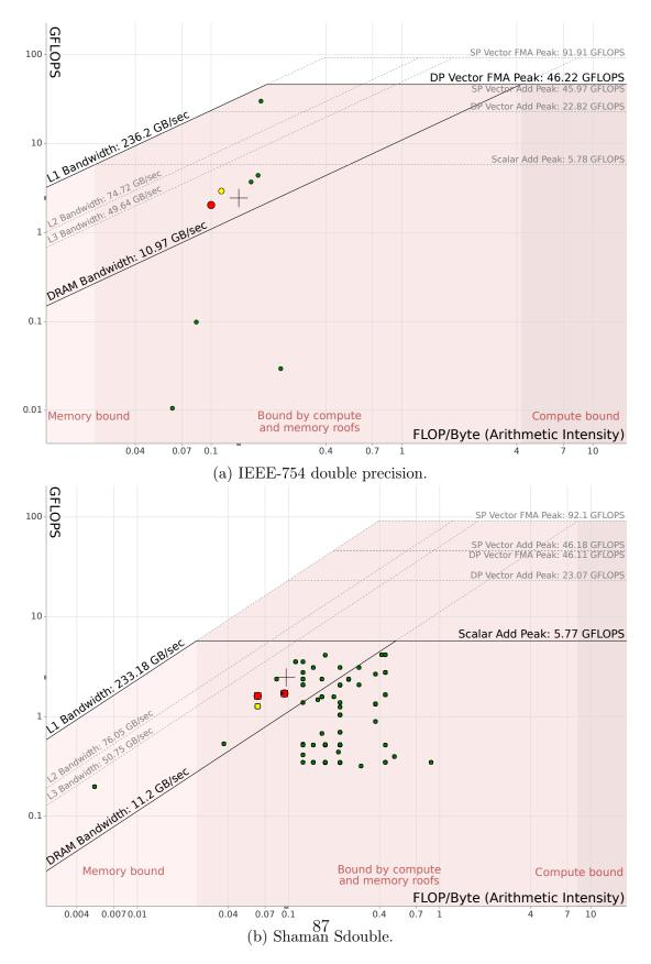
Figure 7.2: Roofline plot comparing the arithmetic intensity of Shaman and double arithmetic on Lulesh 1.0. The x-axis represents the arithmetic intensity while the y-axis is the number of operation per seconds. Green, yellow and red points represent measures, randomly sampled, colored as a function of their associated computing time. Plot produced with Intel advisor [Marques et al., 2017].
