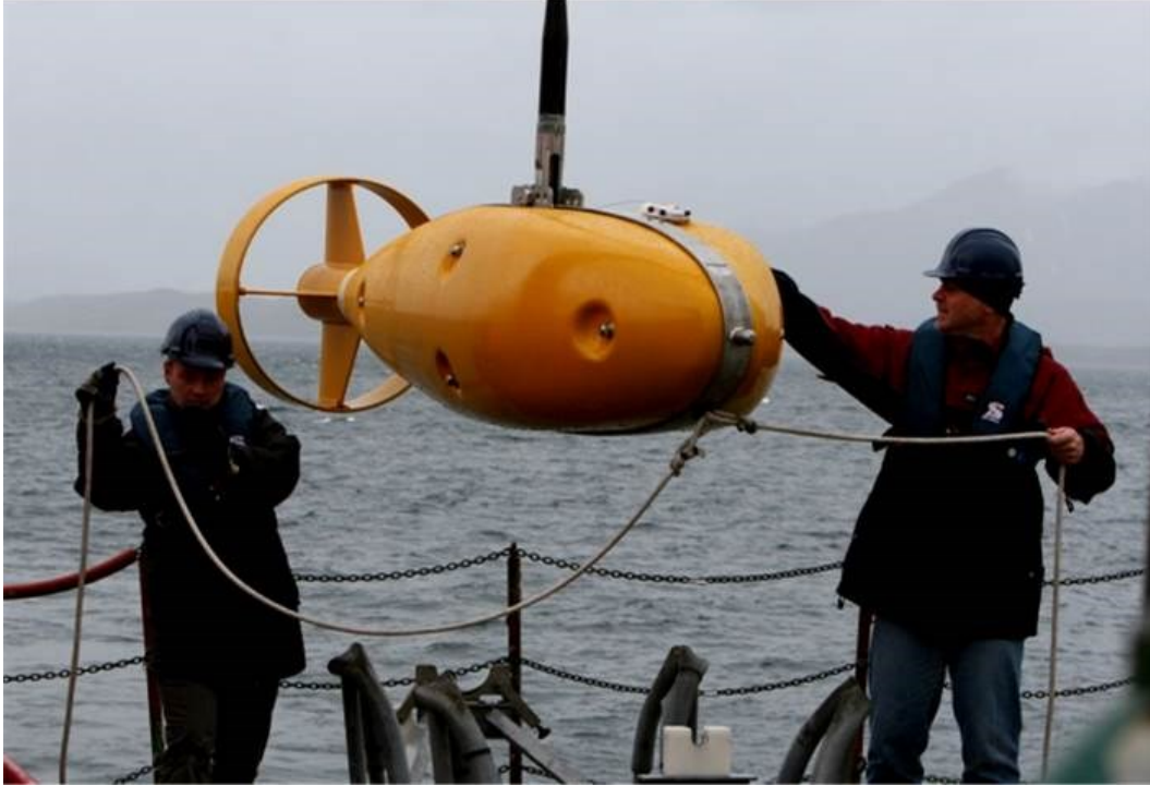
Figure 3: The Socrates towed sonar source used during sonar exposure experiments. Picture credits: 3S project
