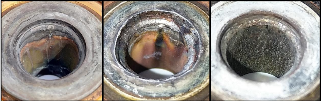
Figure 85 Photos of worn anodes with the arc traces parallel to the torch axis. The anode were used for extended period of time with various parameters (courtesy of Oerlikon Metco (US) Inc.)
