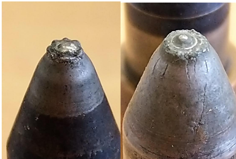
Figure 2: Examples of conic tip cathodes erosion in F4 plasma torch (by courtesy of IRCER, University of Limoges)
