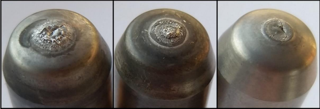
Figure 58 Photos of worn cathodes of the of the SinplexPro™ plasma torch with molten patterns on the top surface. The cathodes were used for extended period of time with various parameters (courtesy of Oerlikon Metco (US) Inc.)
