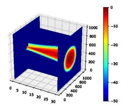
(a) 3D plot of the normalized field (dB) obtained with lSSW.
