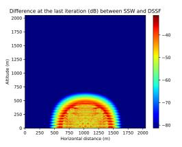
(d) Final normalized difference (dB) between lSSW and DSSF in yOz-plane.
