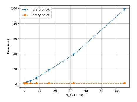
Figure 3.3: Computation time (ms) to obtain the set of propagators with DSSF on the total domain and on  $N_l^{\rm p}$ .
