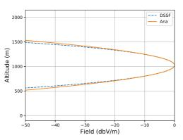
(a) Normalised field (dB) computed with DSSF with  $\Delta z = 0.5$  m.
