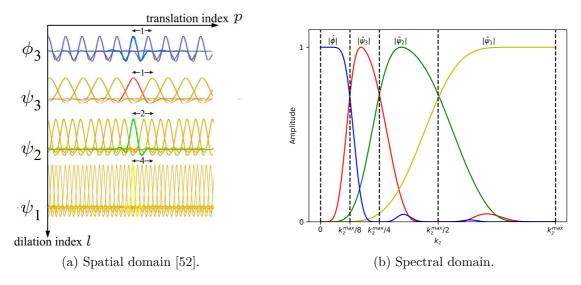
Figure 2.1: Example of a wavelet basis in the spatial domain and of its spectral coverage.
