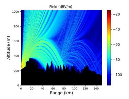
Figure 3.6: Electric field (dBV/m) in the vertical plane obtained by lSSW.
