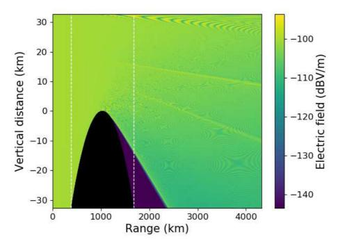
Figure 3.10: Electrical field (dBV/m) obtained with ISSW in scenario 4.
