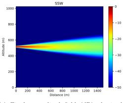
(c) Final normalized field (dB) obtained with lSSW in xOz-plane.
