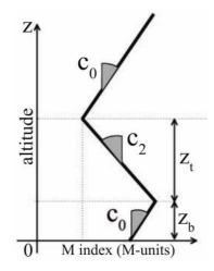
Figure 1.6: Trilinear model of the atmosphere.
