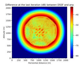
(d) Final normalized difference (dB) between 1SSW and DSSF in yOz-plane
