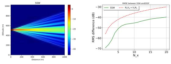
(b) Final normalized field (dB) obtained with lSSW in xOz-plane
