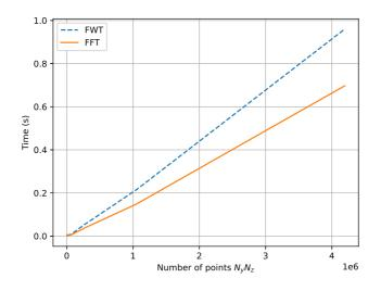
Figure 4.8: Comparison of the computation time of the FFT and the FWT with respect to  $N_y N_z$ .
