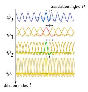
Figure 2.7: Space grid of the wavelets with L = 3 [57].
