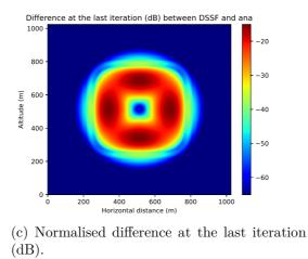
Figure 1.10: Normalised fields obtained at the last iteration with DSSF and compared to the CSP analytical expression in free space.
