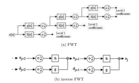
Figure 2.2: Decomposition and recomposition using mirror filters (FWT) [94]
