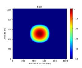
(b) Final normalized field (dB) obtained with lSSW in yOz-plane.
