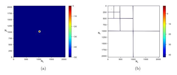
Figure 4.6: Field (dB) radiated from a CSP (a) and its wavelet decomposition (b).
