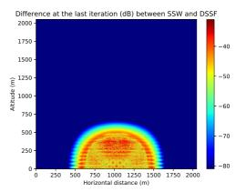
(d) Final normalized difference (dB) between 1SSW and DSSF in yOz-plane.
