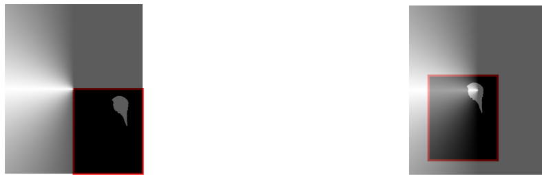
FIGURE 8.2: For each iteration of the fuzzy dilation, D_{SE}(F)(u) with u \in \mathcal{U} , the structuring element SE is looped over the input image F . As shown on these two figures, SE needs to be bigger than F to cover it completely.
