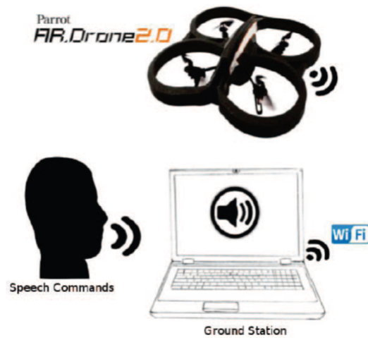
Figure 1.7 – A human operator gives voice commands which are recorded by a microphone and mapped to control commands to a quadrotor [45].
