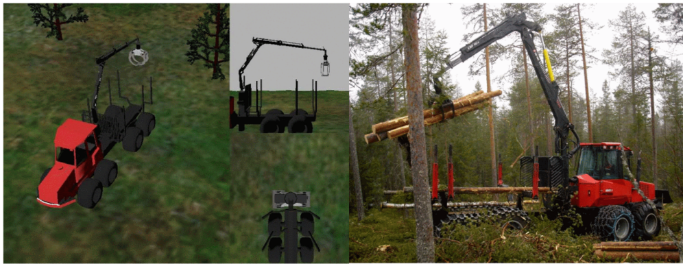
Figure 1.12 – Interface based on virtual environment of a hydraulic crane [65].
