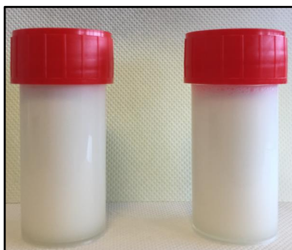
Figure III-9. Macroscopic aspect of O/W (1:3) emulsion stabilized by protein extract from undefatted corn germ
