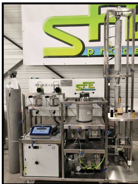
Figure II-7. SFE Lab 2L equipment
