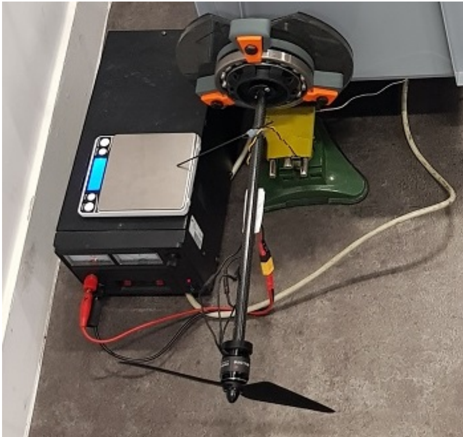
Figure 2.13 – Experimental setup for torque identification of the Tarot 650
