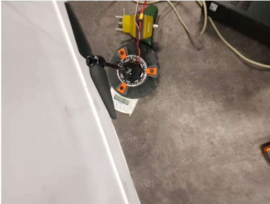
Figure 2.11 – Experimental setup for thrust identification of the Tarot 650
