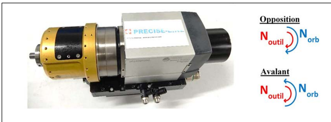
Figure 2.6: Unité de perçage orbital - ORBIBOT (PRECISE France)
