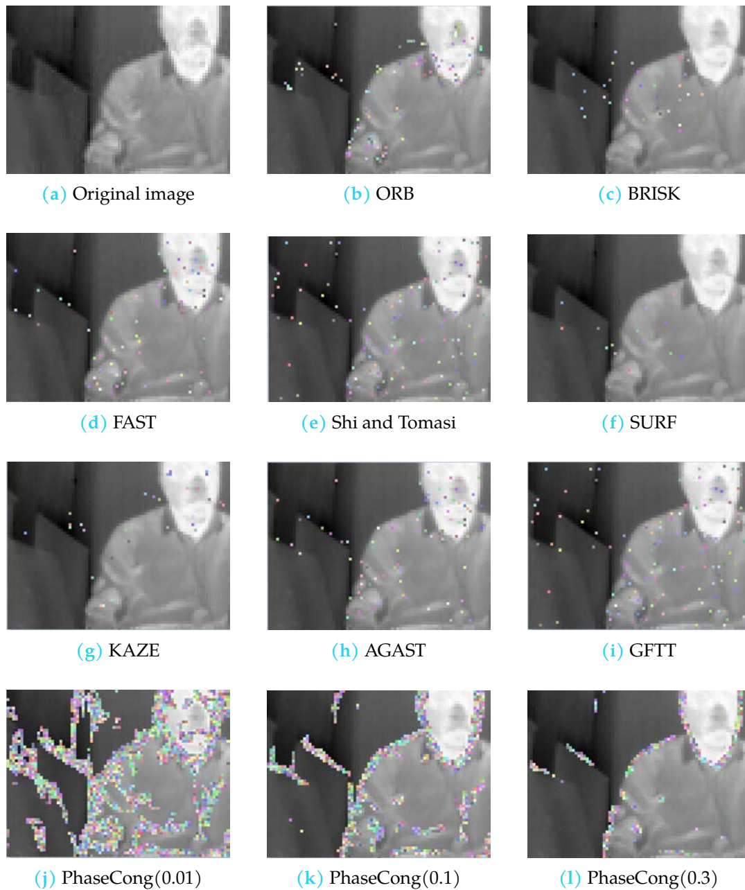
Figure 4.9: Features (colored dots) extracted by several feature extractor methods. The color of feature is generated randomly.
