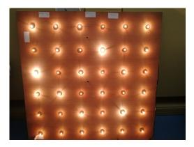
Figure 3.7: Calibration grid
