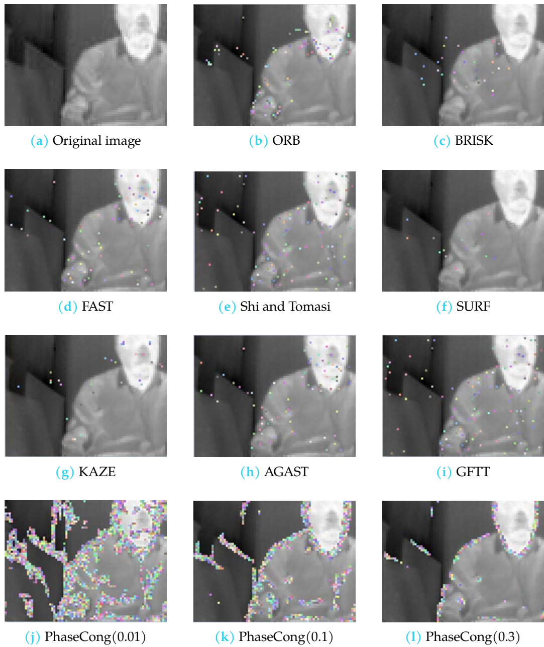
Figure 4.9: Features (colored dots) extracted by several feature extractor methods. The color of feature is generated randomly.
