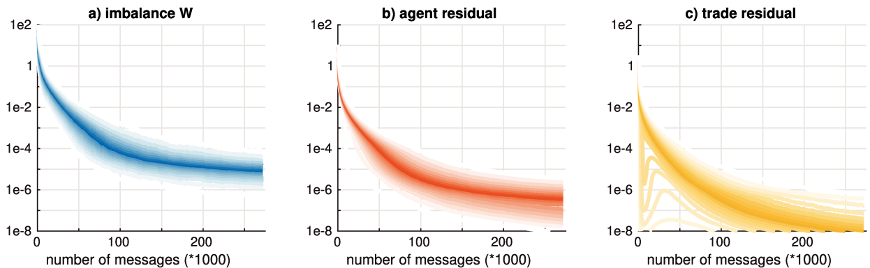
Figure 3.7: Quantiles (5%) of the power imbalance (left), and per prosumer (center) and per trade (right) residuals through messages in a 25 prosumer peer-to-peer market. The total traded volume is 1370 W in this test case.
