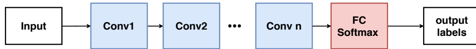
Figure 2.11: In fine-tuning process, all convolutional layers (blue layers) in the network are fixed and gradient is backpropagated through the fully connected (FC) layer only.
