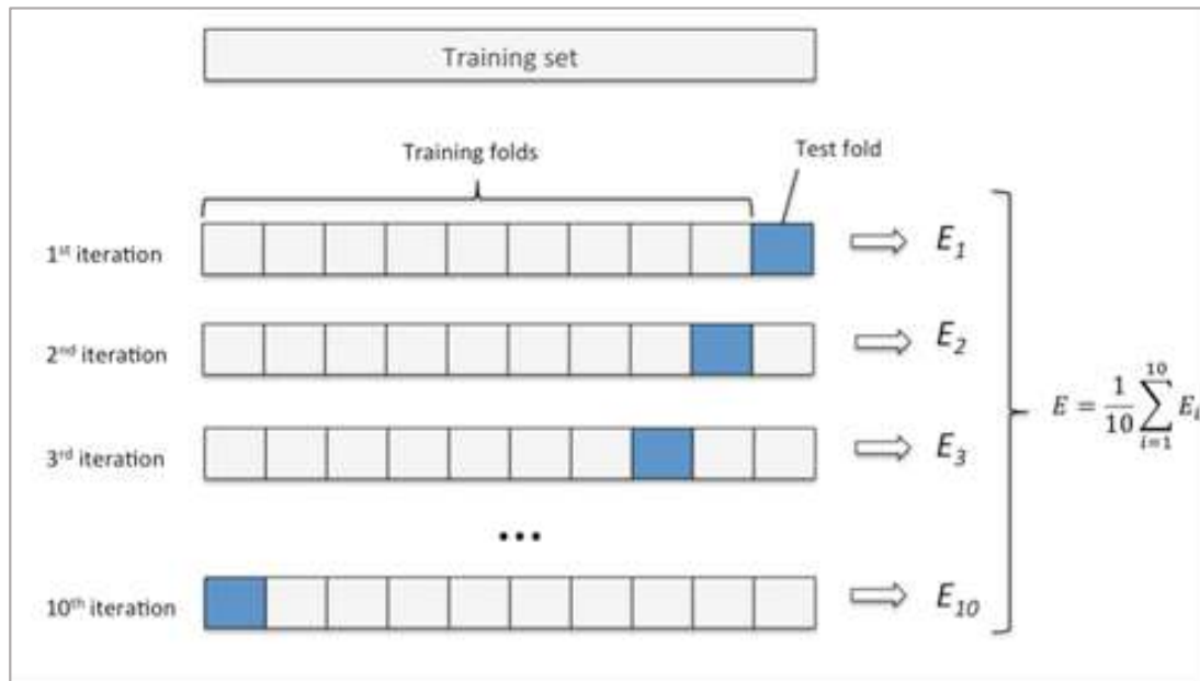
Figure 2.12: 10-fold cross validation. The designated training set is further divided up into K folds ( K=10 ), each of these will now function as a hold-out test set in K iterations. Finally, the scores obtained from the model on individual iterations are summed and averaged into the final score.
