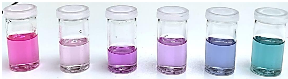
Figure 19. Some deep eutectic solvents in presence of Nile Red. From left to right: TBABr:Dec, ChCl:U, ChCl:EG, ChCl:G, ChCl:Lev and TBPBr:Lev.
