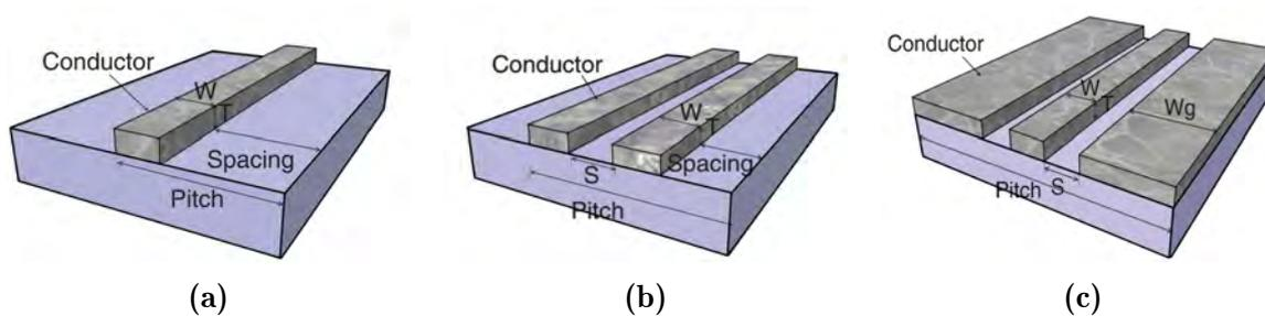
**Figure 1.7:** Three main types of on-chip TLs: (a) microstrip line (MSL), (b) differential line or coplanar strips (CPS), and (c) coplanar waveguide (CPW)
