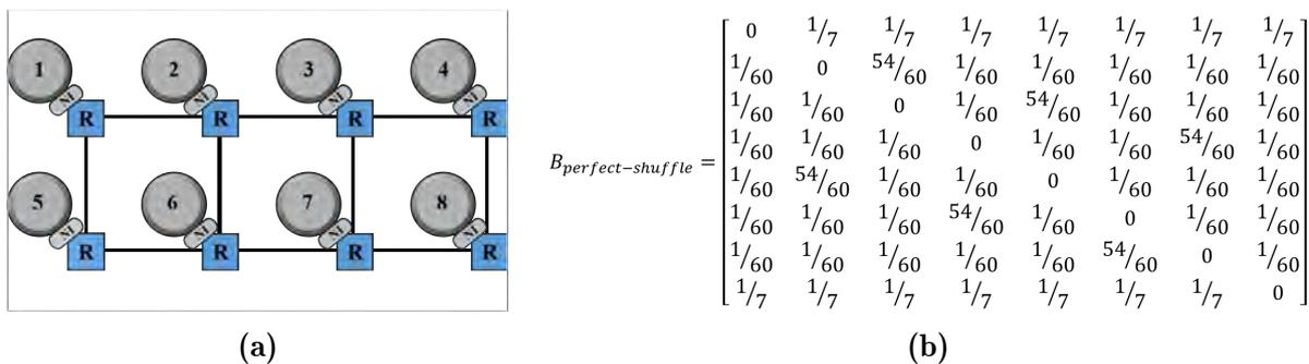
**Figure 5.5:** Example of  $M = 8$  cores with perfect shuffle traffic based on (a) network mesh topology with its respective (b) frequency matrix of communication between cores.
