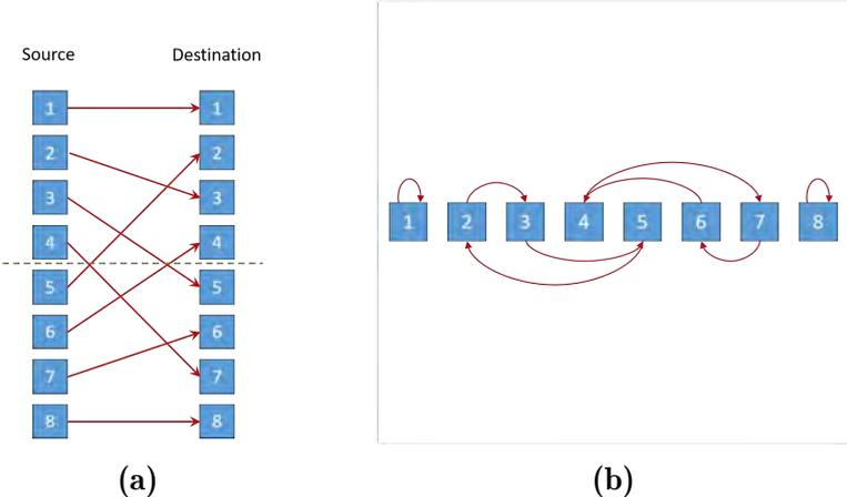
**Figure 5.4:** Example of (a) perfect shuffle for  $M = 8$  cores with the obtained (b) circulating shuffle network.
