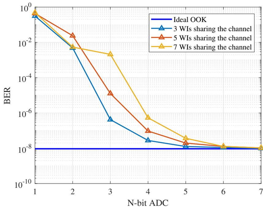
**Figure 2.19:** Average BER for multiple WIs sharing the channel using DSSS with OOK modulation for coherent detection in AWGN channel with QN for different values of  $N$  at  $\text{SNR} = 15$  dB.
