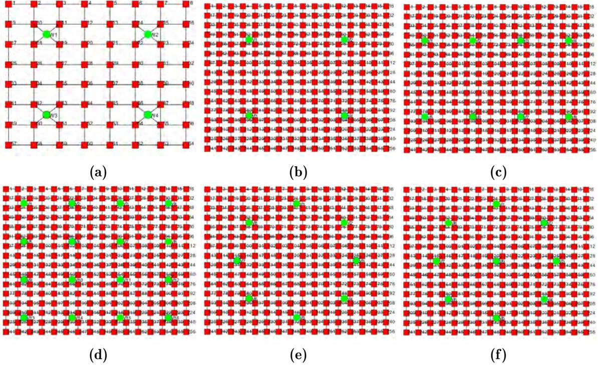
**Figure 5.16:** Antenna placement for evaluation of 64 and 256 cores.
