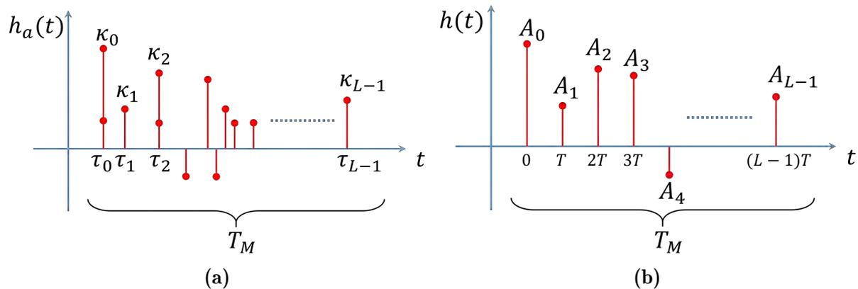
**Figure 2.3:** Representation of the multi-path channel impulse response
