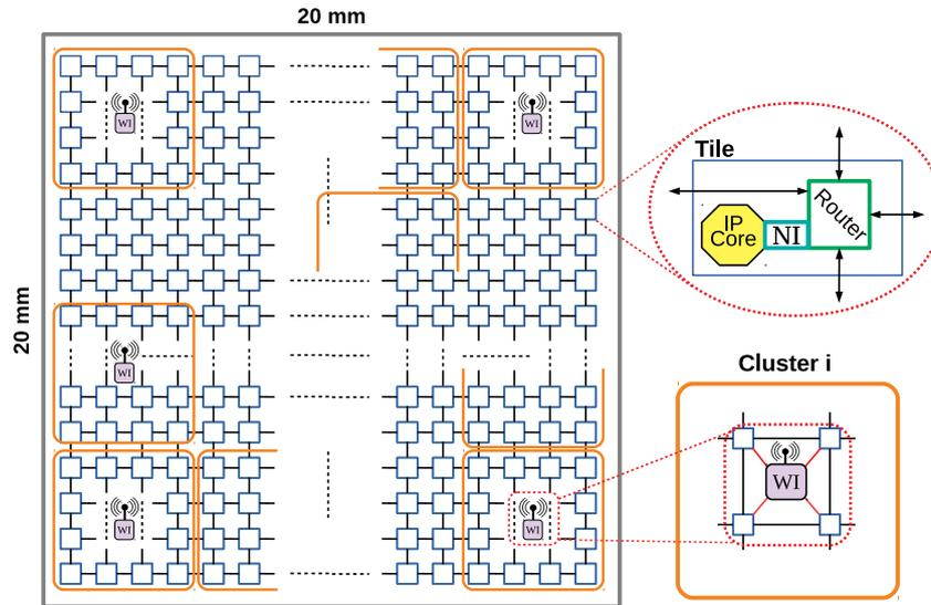
**Figure 3.1:** Wireless interface distribution among a clustered WiNoC hybrid topology with  $N$  clusters of  $M$  cores. The WI of a cluster is connected to four routers.
