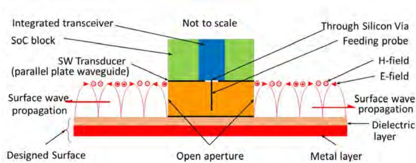
**Figure 1.12:** Integrated transceiver and integrated transducer (inverted quarterwavelength monopole) stacked over a designed surface. [Kar+15]
