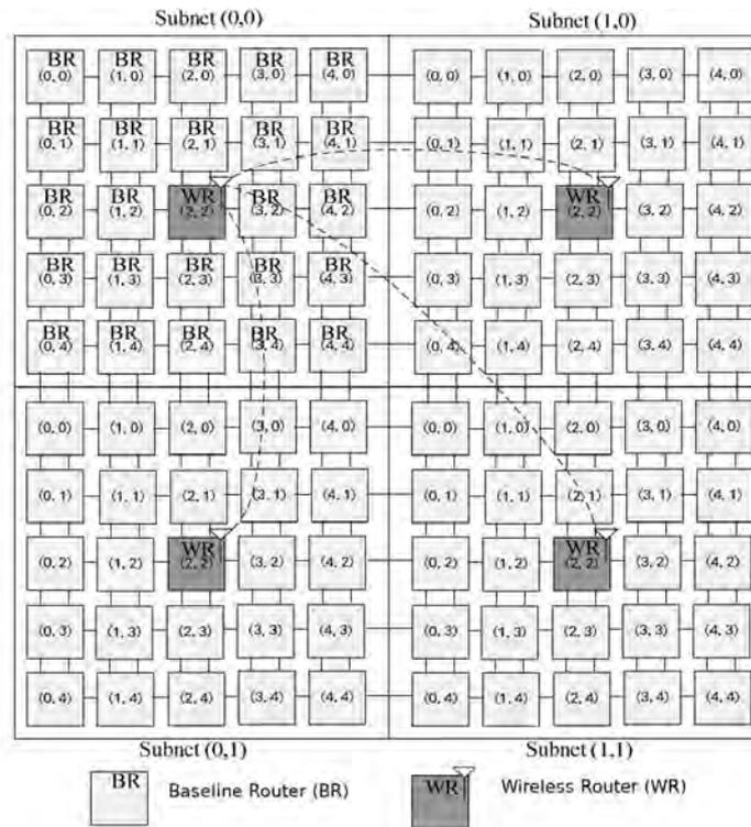
**Figure 1.17:** 2D mesh-based hybrid WiNoC architecture [WHB11]
