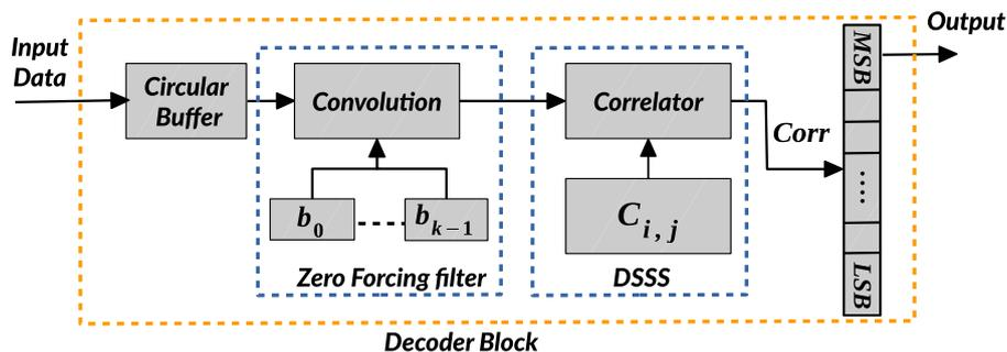
**Figure 2.27:** ZF equalizer with DSSS decoder architecture.
