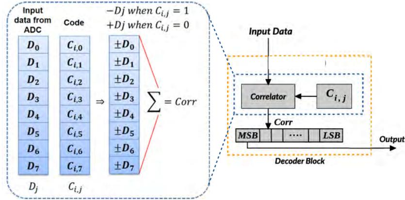
**Figure 2.24:** DSSS decoder architecture.
