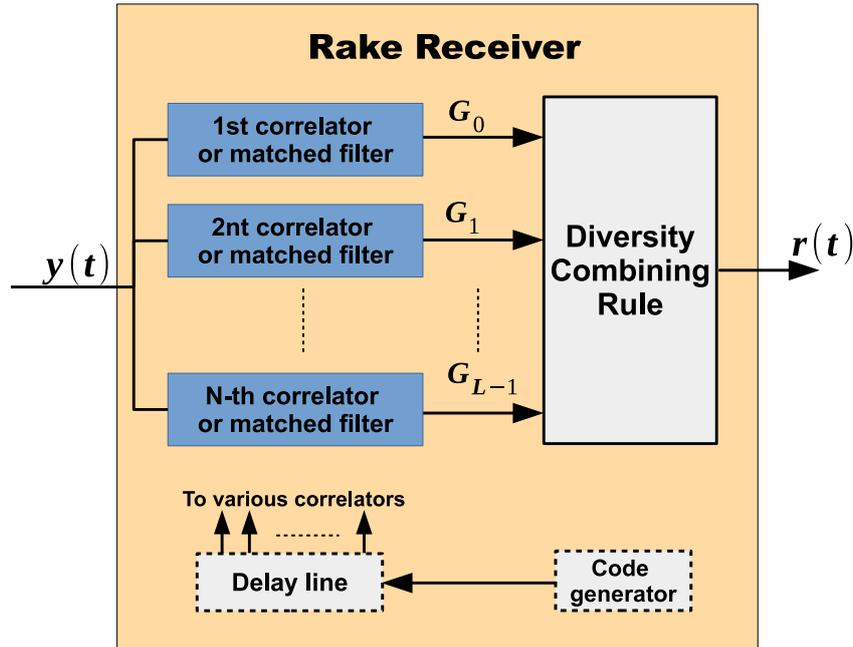
**Figure 2.20:** Diversity demodulator for spread-spectrum signals over multi-path channels.
