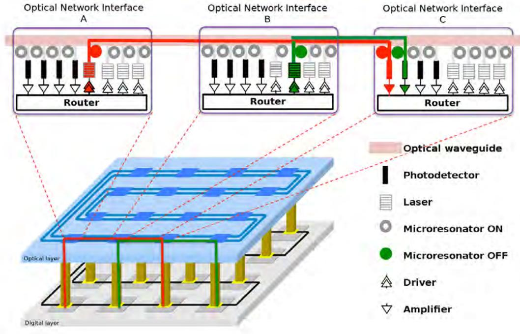
**Figure 1.6:** Conventional optical network interface architecture [Chi+17]
