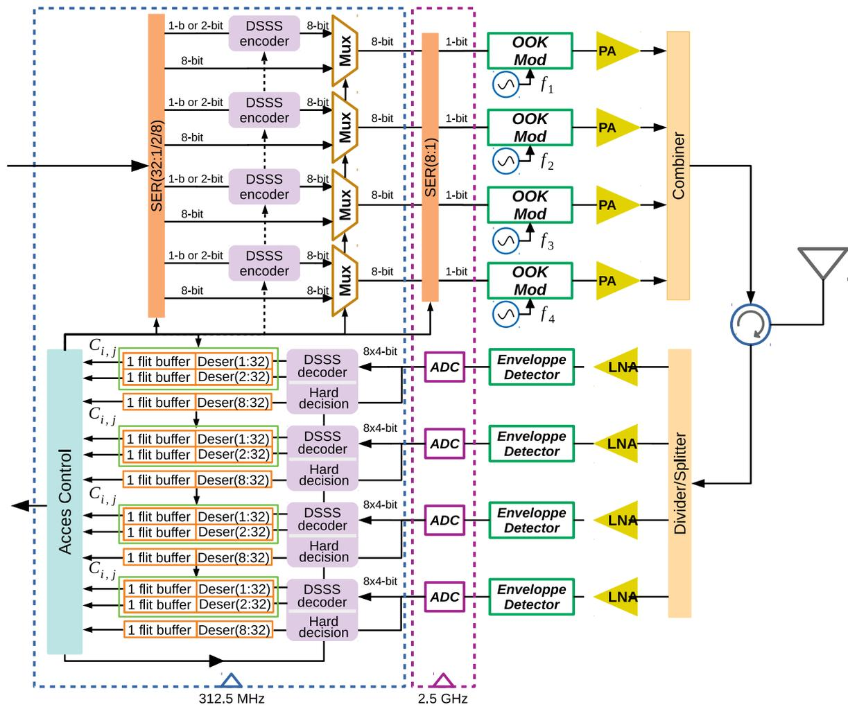
Figure 4.7: Enhanced digital-domain transceiver architecture.
