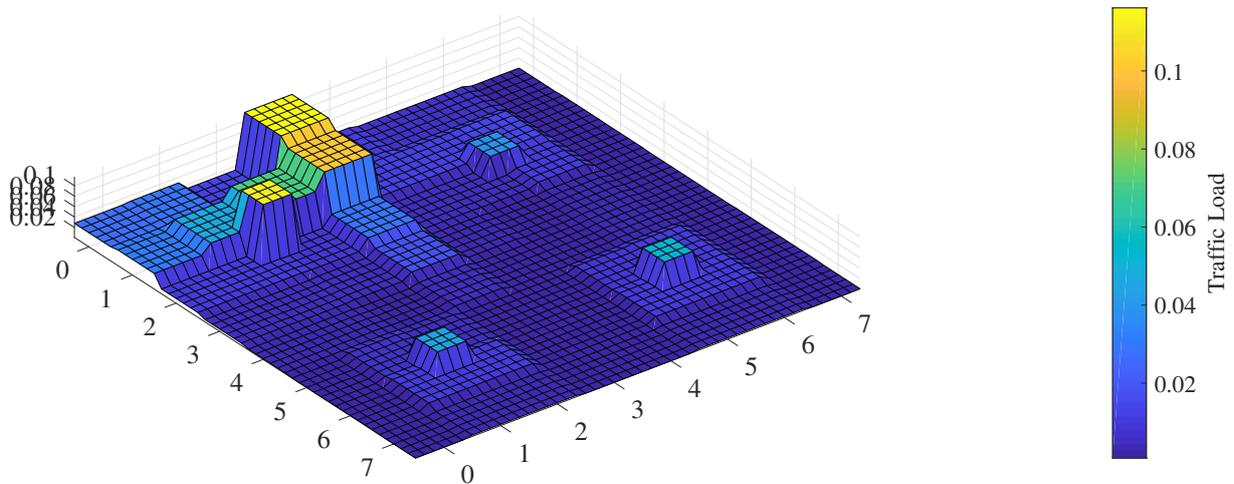
**Figure 5.18:** Network behaviour generated by application benchmark x264 into a 64-core WiNoC using 4 antennas rectangularly placed into the chip.
