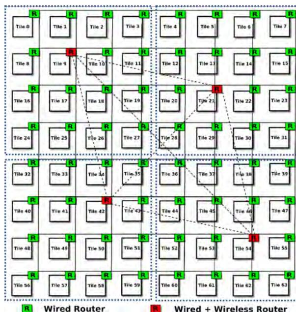
**Figure 1.18:** 2D mesh-based hybrid WiNoC architecture [SD16]
