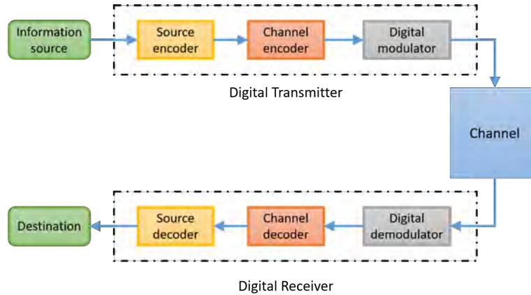
**Figure 2.1:** Block diagram of a digital communication system
