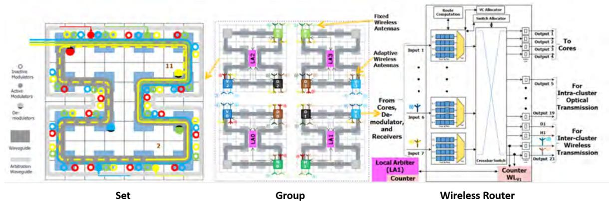
**Figure 1.21:** Optical-Wireless Network-on-Chip architecture [SKL16]
